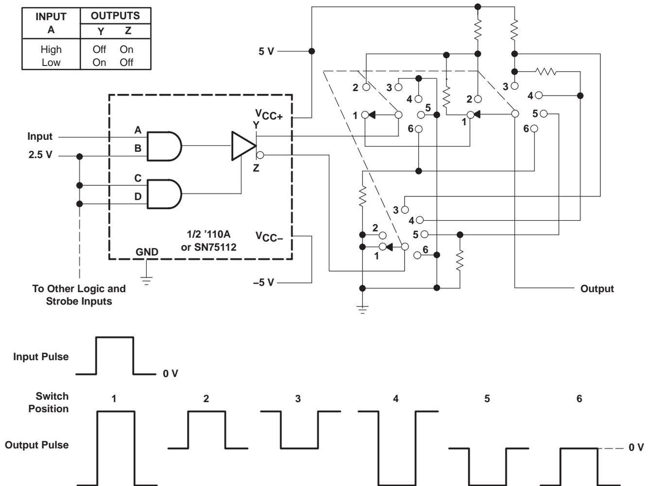
Figure 4. Pulse-Control Circuit
