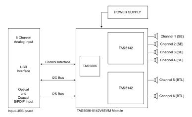
Figure 1-1. Integrated PurePath Digital™ Amplifier System
