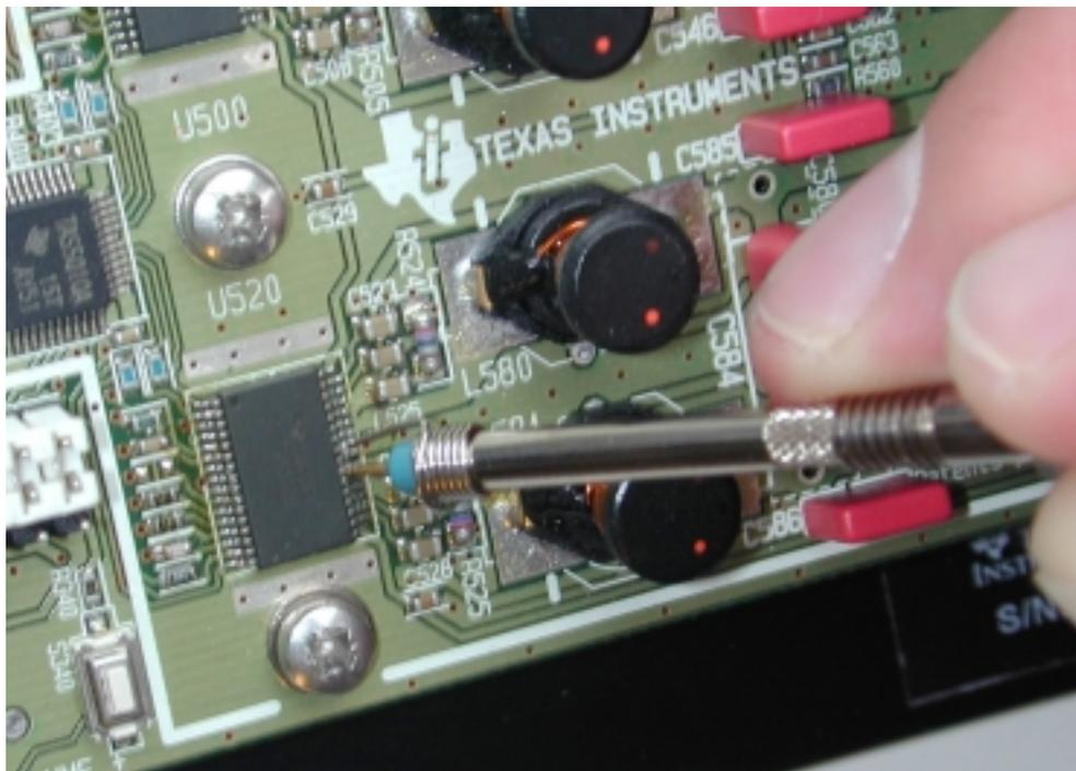
**Figure 4 Probe as close to the pin as possible**
