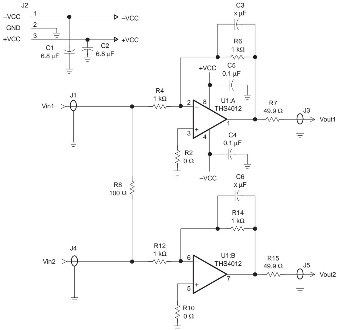
The gain of the EVM inputs can easily be changed to support a particular application by changing the ratio of resistors R6 and R4 (channel 1) and R14 and R12 (channel 2) as described in the following equation:
