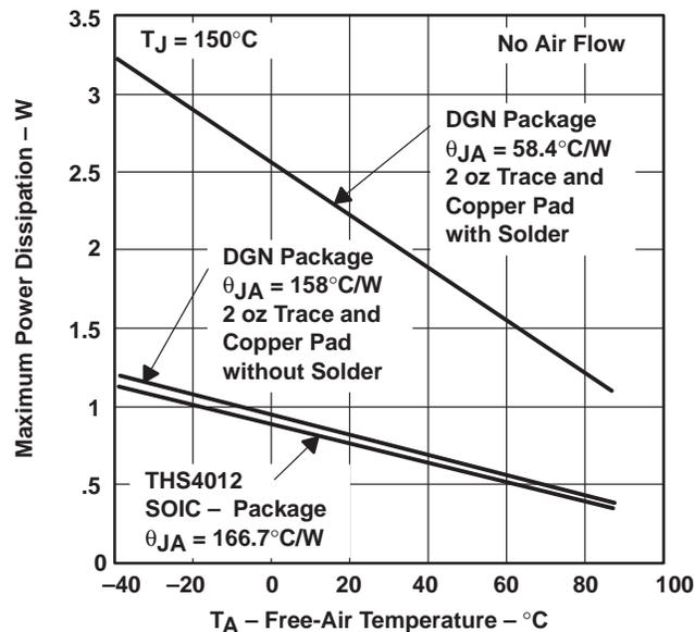
Even though the THS4012 EVM PCB is smaller than the one in the example above, the results should give an idea of how much power can be dissipated by the PowerPAD IC package. The THS4012 EVM is a good example of proper thermal management when using PowerPAD-mounted devices.
