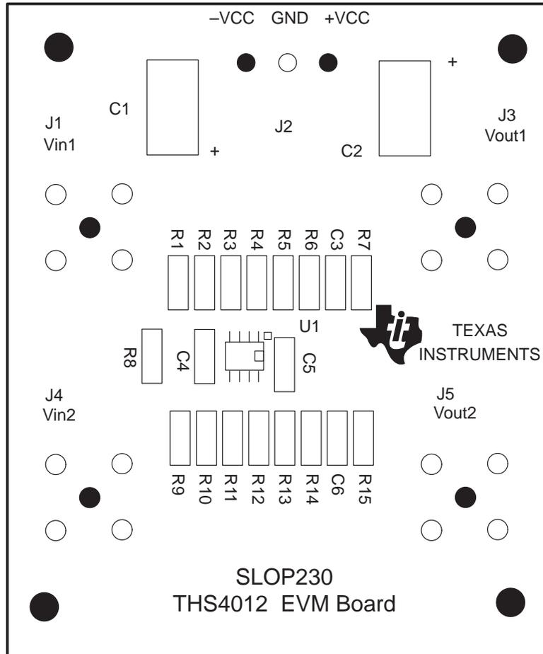
Figure 2–3. THS4012 EVM PC Board Layout – Component Side
