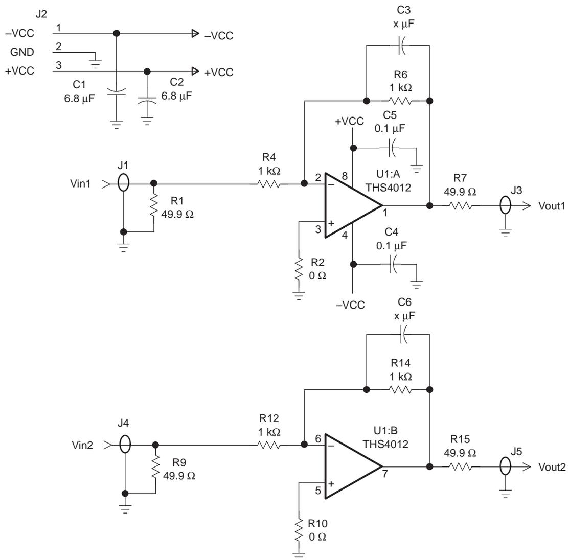
The gain of the EVM can easily be changed to support a particular application by changing the ratio of resistors R6 and R4 (channel 1) and R14 and R12 (channel 2) as described in the following equation:
