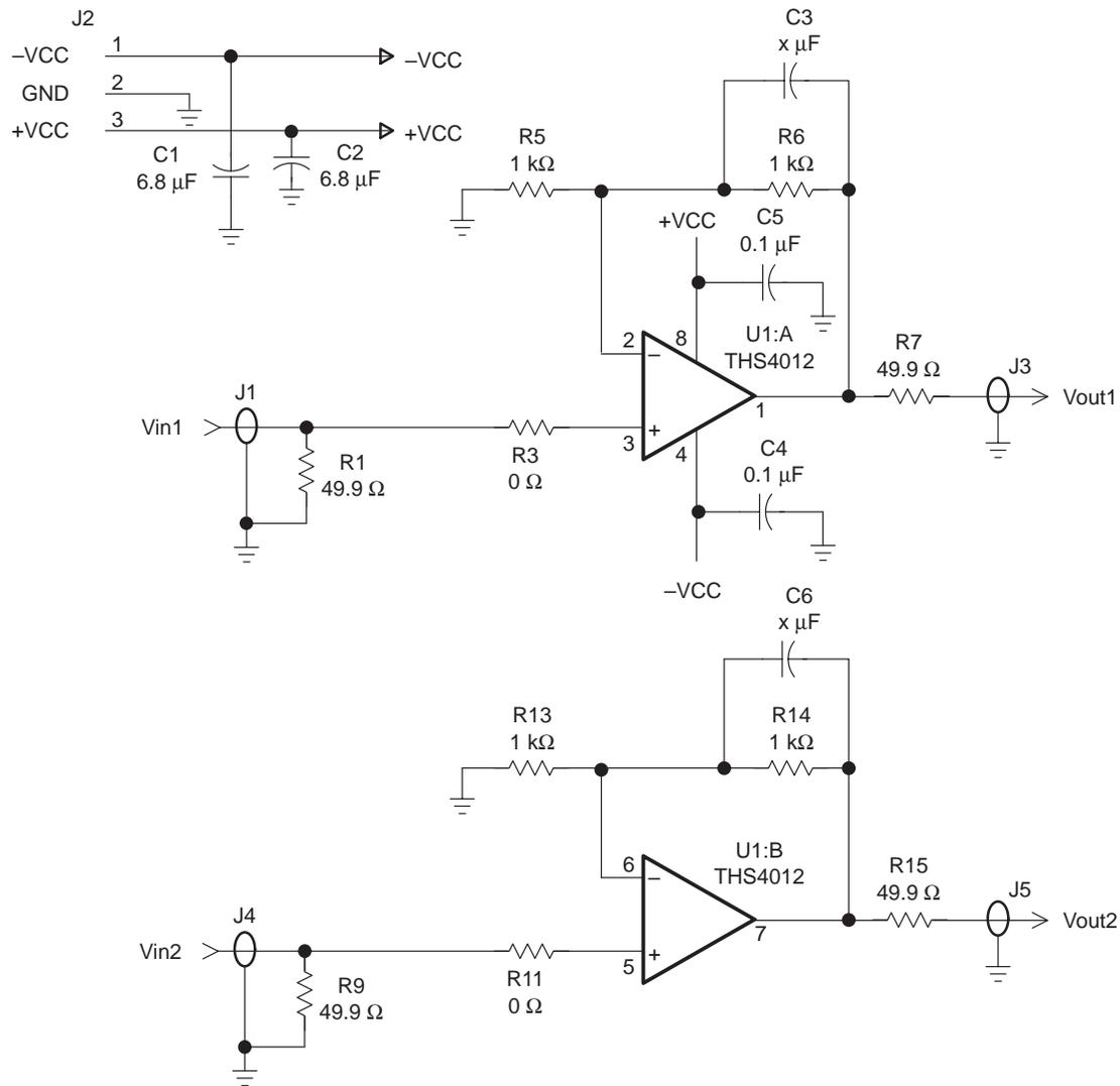
The gain of the EVM can easily be changed to support a particular application by simply changing the ratio of resistors R6 and R5 (channel 1) and R14 and R13 (channel 2) as described in the following equation:
