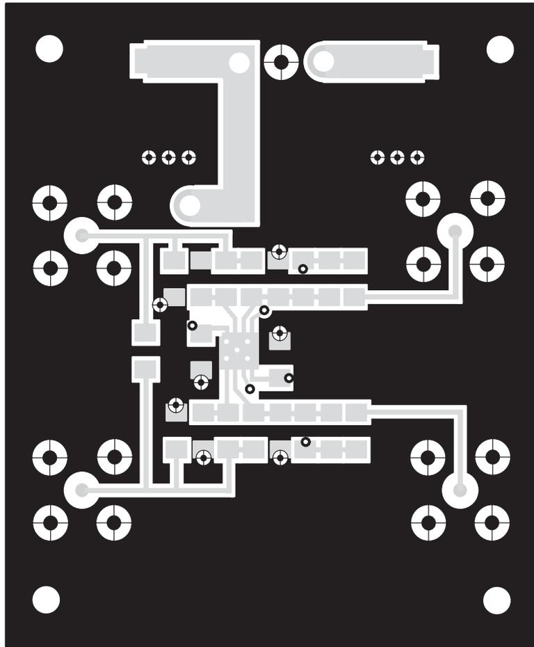
Figure 2–4. THS4012 EVM PC Board Layout – Back Side
