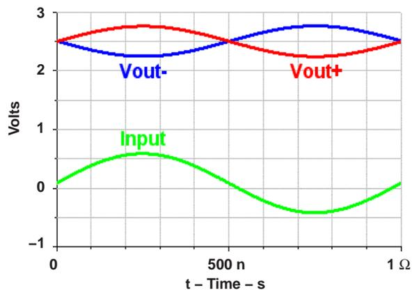
Note that a small offset is present on the input voltage. This is caused by a voltage divider formed by  $R_2 + R_4$  and the parallel combination of  $R_1$  and the source resistance of the signal generator.
