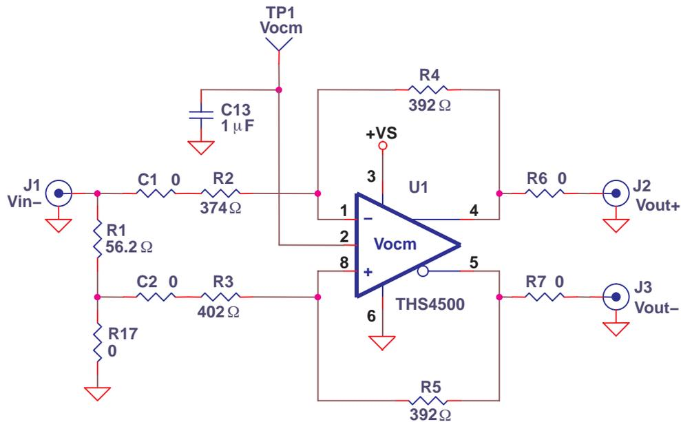
Figure 3–3. Output of an AC-Coupled, Single-Supply Application
