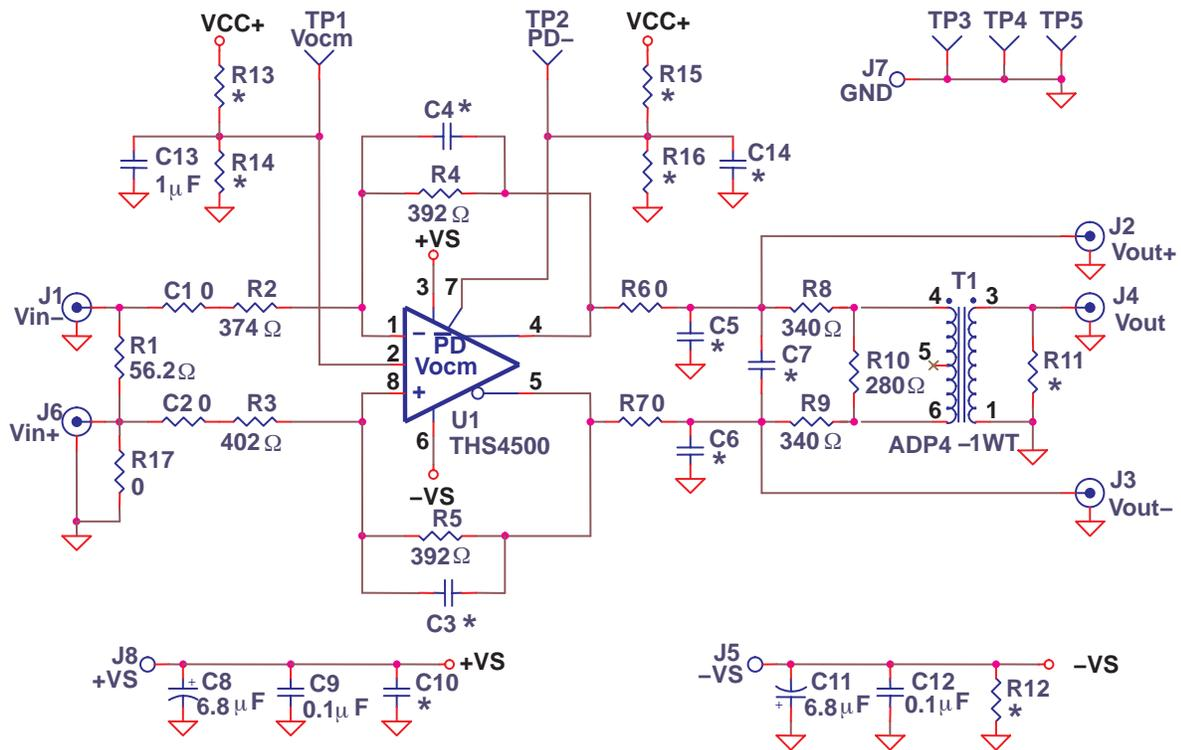
**Note:** Devices designated with an \* are not installed on the EVM. The user must supply these components.
