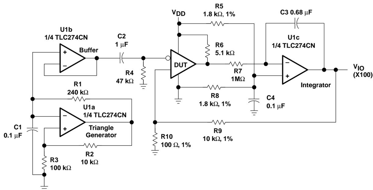
**Figure 2. Circuit for Input Offset Voltage Measurement**
