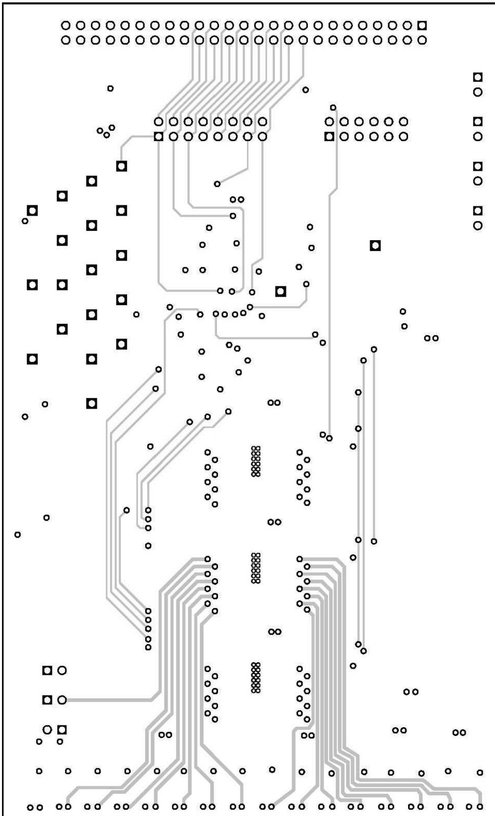
Figure 5. Layer 3 Routing
