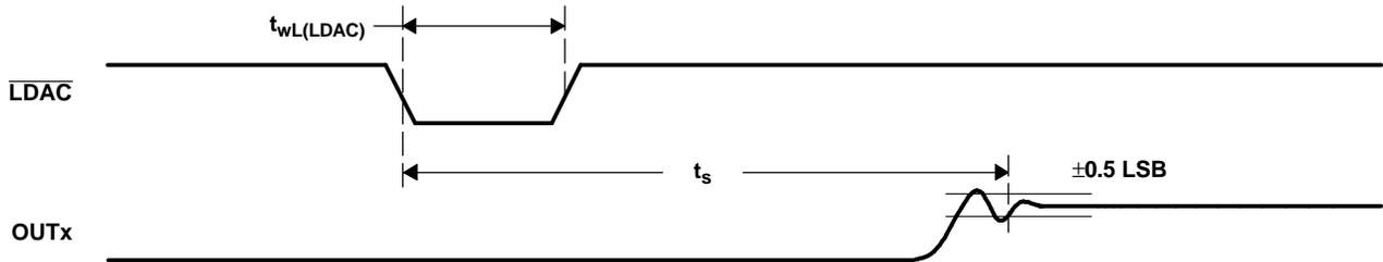
**Figure 12. Output Timing**
