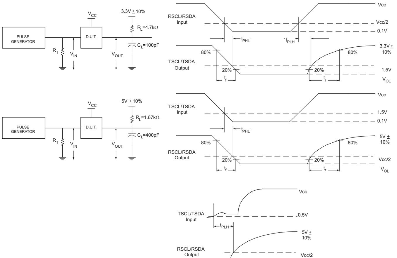
Figure 9. I<sup>2</sup>C Timing Test Circuit and Definition
