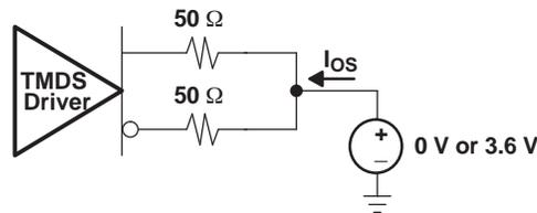
Figure 5. Short Circuit Output Current Test Circuit
