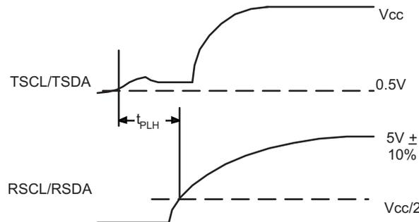
**Figure 20. Waveform of Turning Driver T Off**
