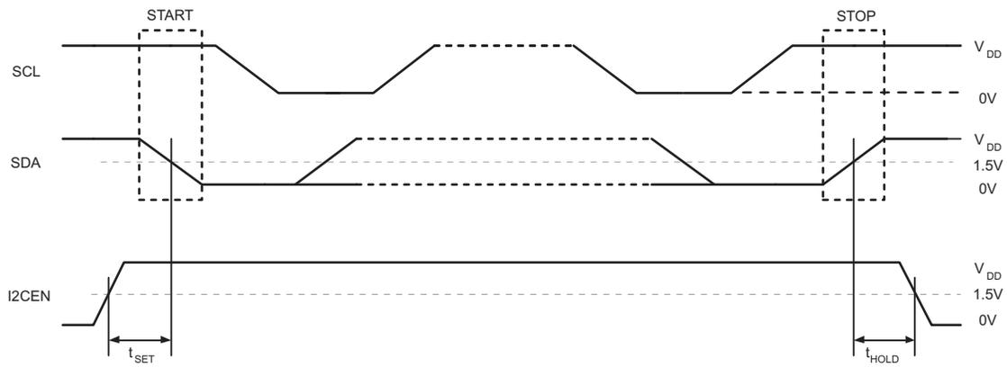
**Figure 10. I<sup>2</sup>C Setup and Hold Definition**
