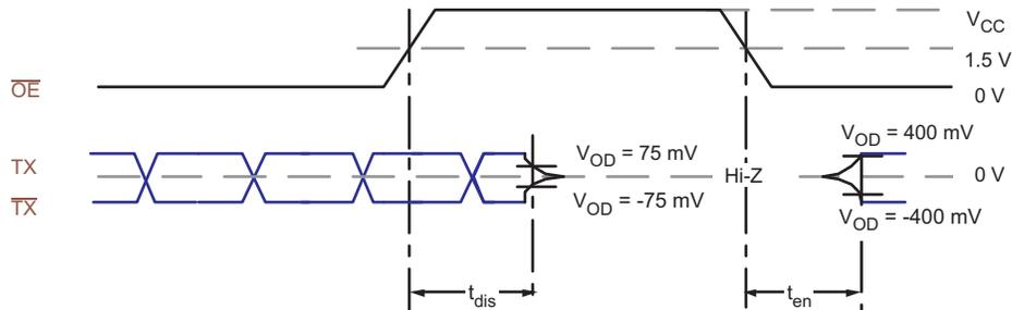
Figure 7. TMDS Enable and Disable Timing Definitions
