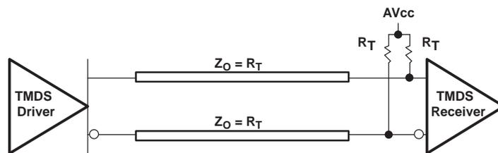
Figure 2. Typical Termination for TMDS Output Driver
