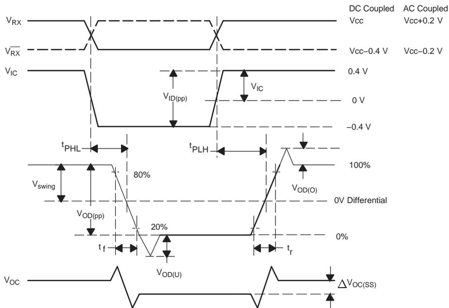
NOTE: PRE = low. All input pulses are supplied by a generator having the following characteristics:  $t_r$  or  $t_f < 100\text{ ps}$ , 100 MHz from Agilent 81250.  $C_L$  includes instrumentation and fixture capacitance within 0.06 m of the D.U.T. Measurement equipment provides a bandwidth of 20 GHz minimum.
