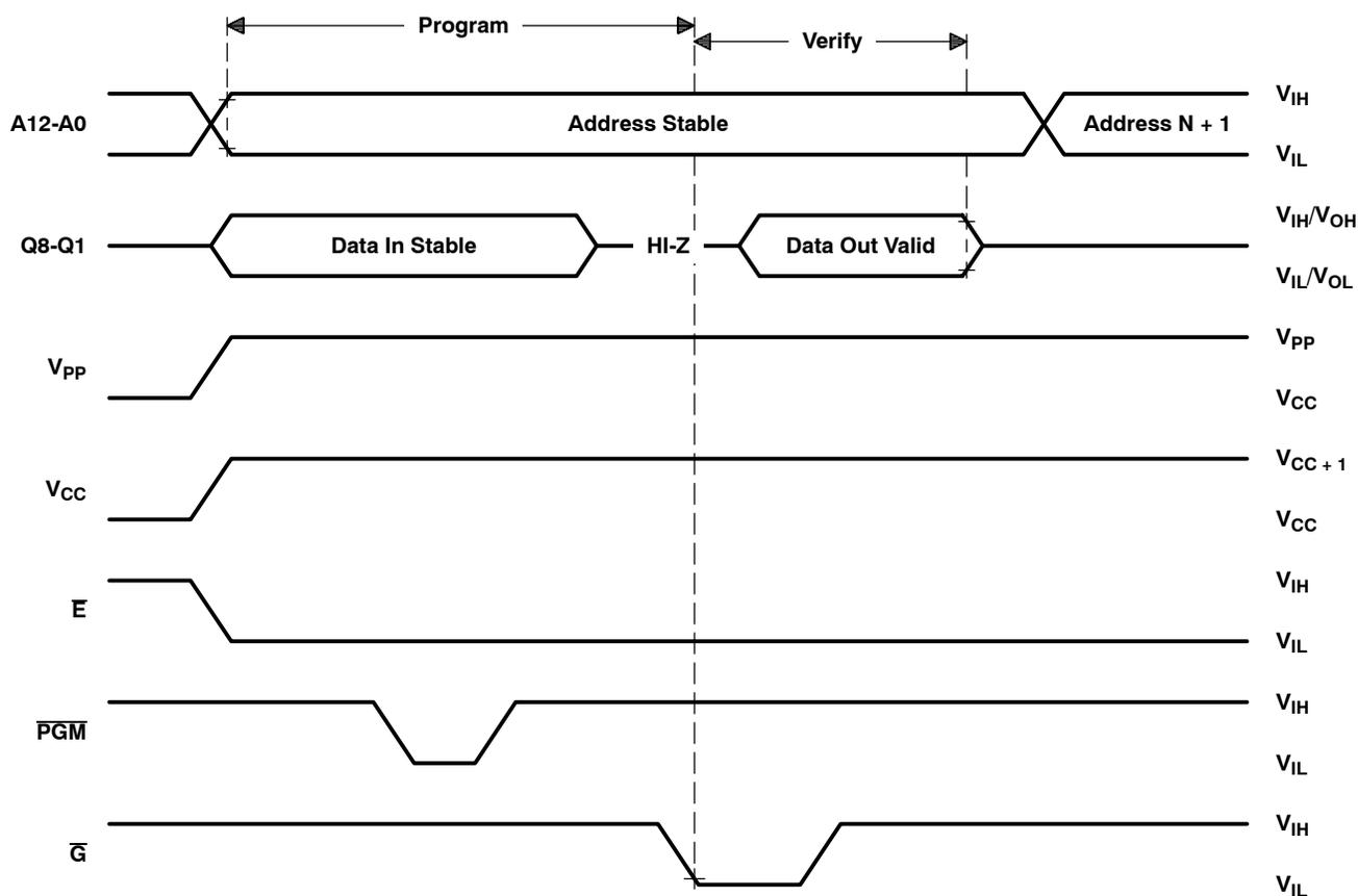
Figure 11. Fast Programming Timing
