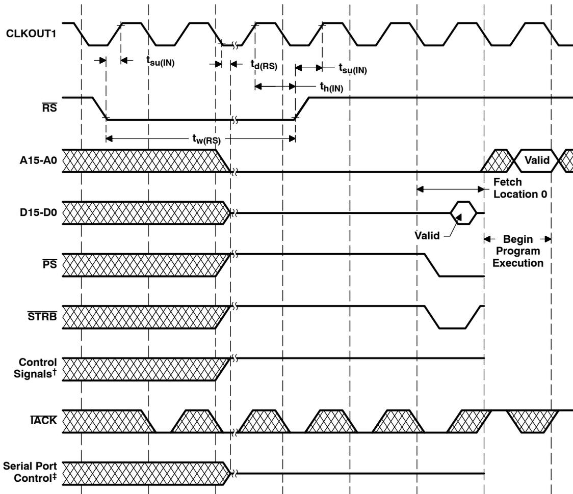
† Control signals are  $\overline{DS}$ ,  $\overline{IS}$ , R/W, and XF.
