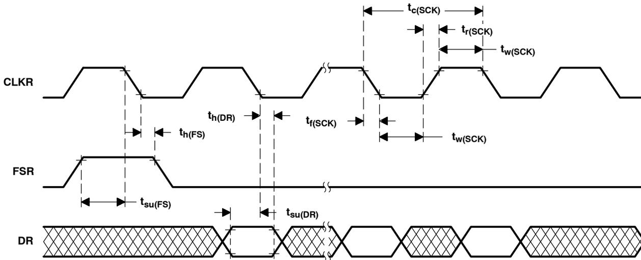
serial port transmit timing
