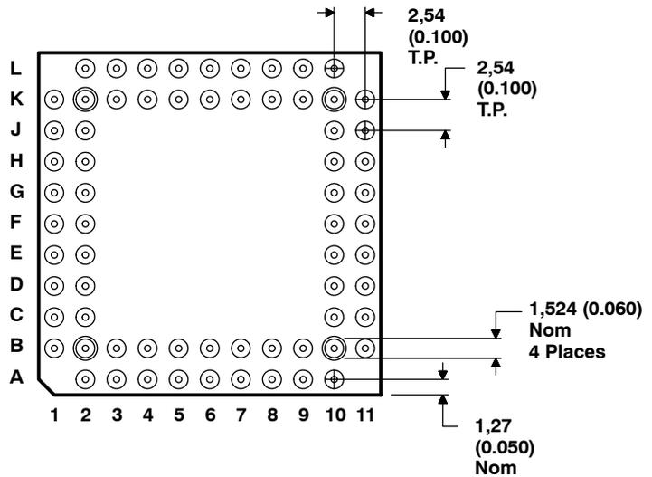
ALL LINEAR DIMENSIONS ARE IN MILLIMETERS AND PARENTHETICALLY IN INCHES
