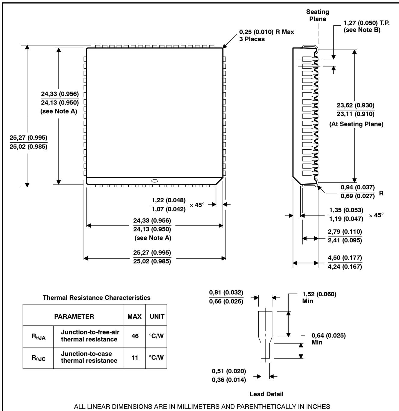
NOTES: A. Centerline of center pin, each side, is within 0,10 (0.004) of package centerline as determined by this dimension.
