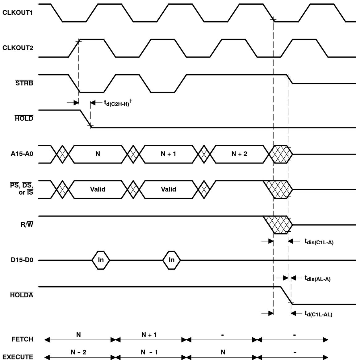
†  $\overline{\text{HOLD}}$  is an asynchronous input and can occur at any time during a clock cycle. If the specified timing is met, the exact sequence shown will occur; otherwise, a delay of one CLKOUT2 cycle will occur.
