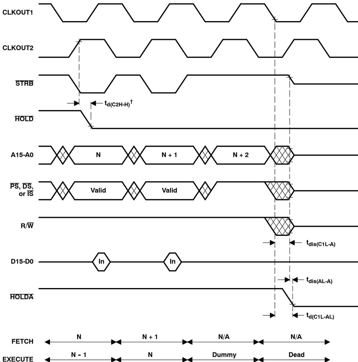
$^\dagger$   $\overline{\text{HOLD}}$  is an asynchronous input and can occur at any time during a clock cycle. If the specified timing is met, the exact sequence shown will occur; otherwise, a delay of one CLKOUT2 cycle will occur.
