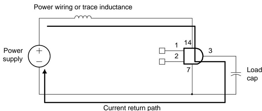
**Figure 4-2. Power Supply Current Return Path Example 2**
