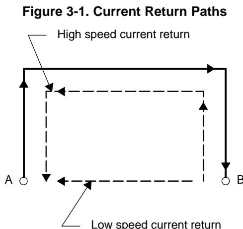
The current return density and the amount of crosstalk can be estimated as shown in [Figure 3-2](#) and [Figure 3-3](#). Based on the equations shown in the figures, the spacing between the traces and the distance that they run in parallel determines the amount of crosstalk. Obviously, moving the traces further from each other will reduce the crosstalk.
