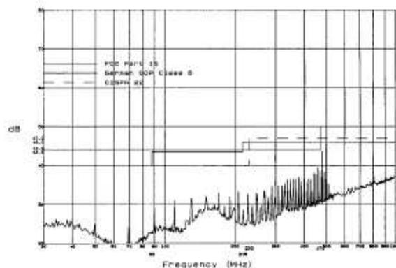
Radiated Emissions from PCB With Image Plane
