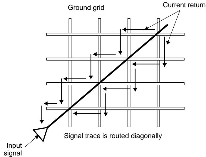
So, if ground grid is a required in a design, the best approach is to route the high speed signals right on top of the grids and parallel to the grid to ensure the smallest current return loops. This lowers the characteristic impedance to the level equivalent to the impedance of the continuous ground plane. This is very difficult to accomplish since complex board has many high speed traces. Therefore, continuous ground plane is still the best method to keep characteristic impedance and EMI low.
