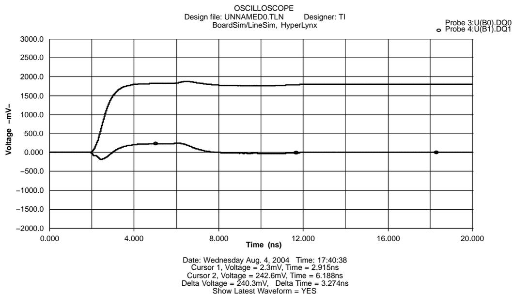
Figure 3-5 shows simulation results. On the victim trace, the first negative-going pulse, which has a  $-200\text{mV}$  peak, is the forward crosstalk. The positive-going pulse of  $240\text{mV}$  is the backward crosstalk. The backward pulse width is about 2 times the coupling region. In this case, the coupling region is  $3.54\text{nS}$  and the simulation shows a  $4\text{nS}$  backward crosstalk pulse.
