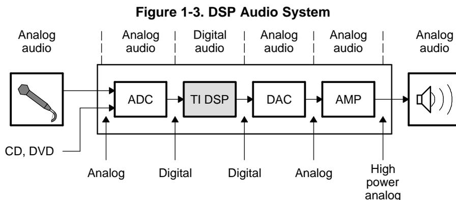
All of the blocks shown in [Figure 1-3](#) from the ADC to the Amp stage are very sensitive to noise so any interference coupled to any of the blocks will propagate and generate unwanted audible sounds. Common audio design problems include:
