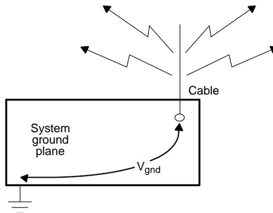
The electric field generated by common radiation is directly related to the frequency propagating on the cable, the length of the cable, and the current driving the cable. Here is an equation to calculate the common mode radiation in an open field.
