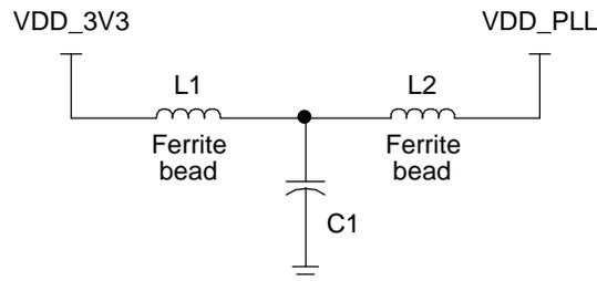
A T filter consists of two ferrite beads and one capacitor as shown in Figure 6-8. Just like in a Pi filter, 3.3V supply noise is attenuated by the L1 ferrite bead and the C1 capacitor and PLL noise is isolated by the L2 ferrite bead and C1 capacitor. The equations are as follows.
