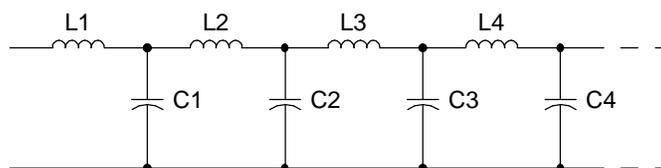
The speed of the signal,  $V_p$ , is dependant on properties such as characteristic impedance,  $Z_o$ , which is defined as an initial voltage  $V^+$  divided by the initial current  $I^+$  at some instant of time. The equations for  $V_p$  and  $Z_o$  are:
