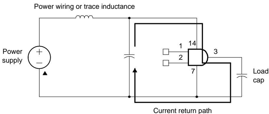
One of the most challenging tasks for system designers is determining an acceptable noise level for a DSP in a particular application. DSP data manuals clearly specify the operating conditions but cannot account for the dynamic nature of high-speed systems. This is because the dynamic switching characteristics very much depend upon on the actual system design and layout. The following are some of the important issues that must be addressed during the power supply design process:
