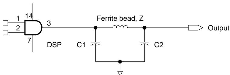
**Figure 4-15. T Filter Circuit for High Speed Signals**
