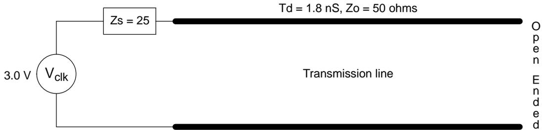
$$V_{initial} = V_{clk} \frac{Z_o}{Z_s + Z_o} = 3 \frac{50}{25 + 50} = 2V$$
