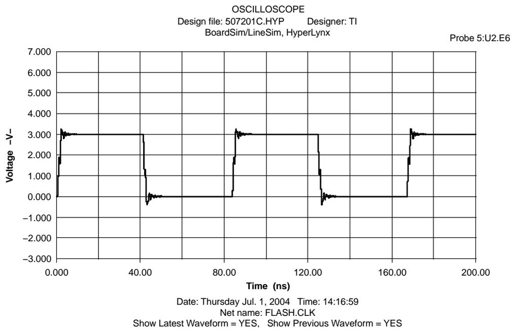
Figure 2-12. Lab Measurement of FLASH.CLK
