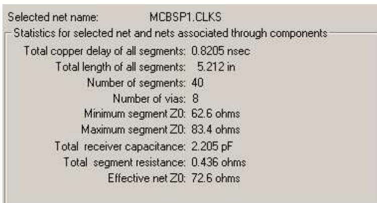
Figure 2-14 shows an audio clock that transmits by U17 and receives by U3. The design has a 20-ohm series termination resistor but no parallel termination at the load. This demonstrates the concept discussed earlier.
