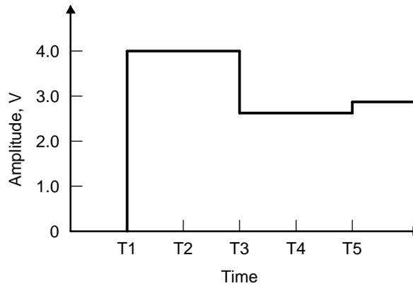
As shown in the example, the reflections with a 3V source caused the signal to overshoot as high as 4V at the load as explained below:
