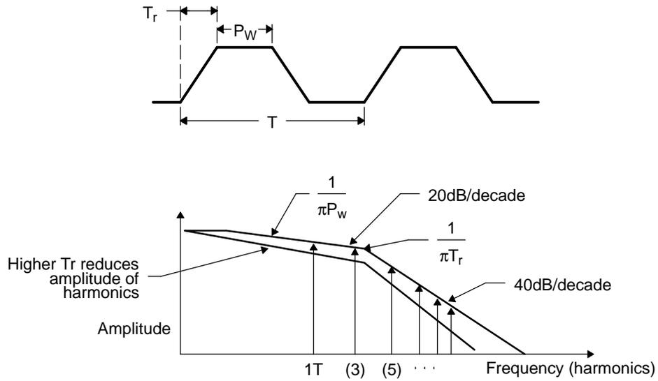
**Figure 3-8. Clock Harmonic Interfered with Video**
