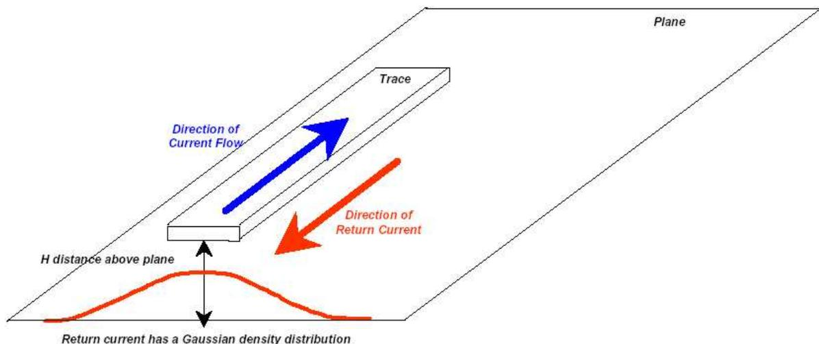
If the ground plane is not continuous underneath the high speed signal, all, crosstalk, reflections and EMI, will increase because of the impedance mismatch and larger current loop return area as shown in [Figure 7-7](#).
