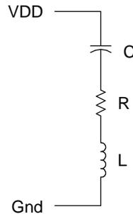
The series equivalent circuit for a capacitor has three different components, equivalent series resistance (ESR), equivalent series inductance (ESL) and the capacitance itself. The self-resonant frequency happens at the point where the impedance of the capacitor, C, is equal to the impedance of the inductor, L.
