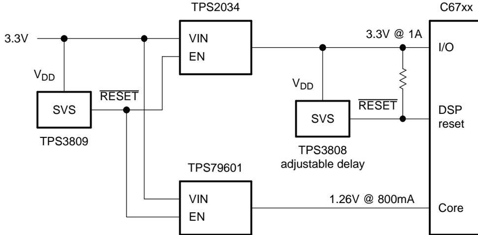
**Figure 4-4. Core Before IO Example**
