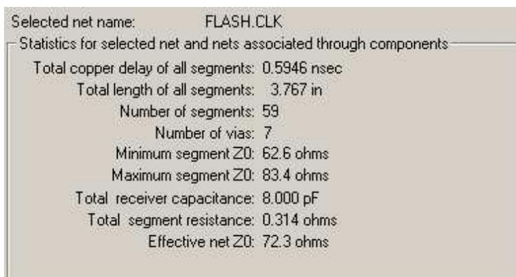
The selected signal is FLASH.CLK which is a clock signal generated by a TI DSP. [Figure 2-10](#) shows an actual PC board designed with one of the TI DSPs where the clock is driven by U3 and is measured at U2.
