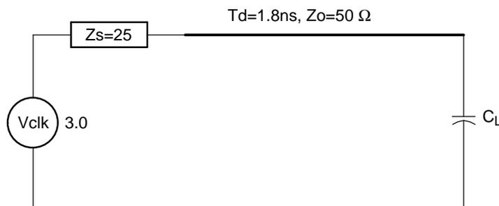
In [Figure 2-8](#), the voltage at the load is slowly charged up to the maximum amplitude of the clock signal. Initially, the load looks like a short circuit. Once the capacitor is fully charged, the load becomes an open circuit. The source resistor  $Z_s$  controls the rise and fall times. Higher source resistance yields slower rise time. The load voltage at any instant of time,  $t$ , greater than the propagation delay time, can be calculated using the following equation:
