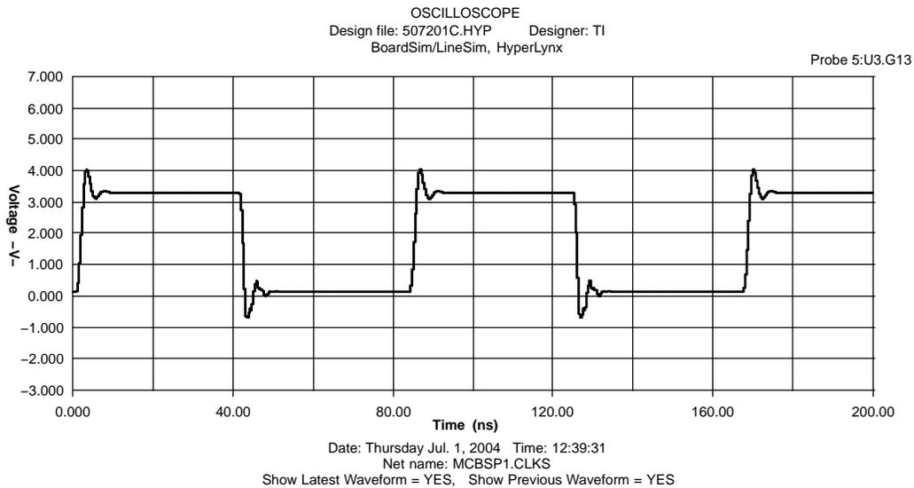
The lab measurement shown in [Figure 2-16](#) correlates with the Hyperlynx simulation very well. The 22-ohm series resistor can be modified to lower the overshoots and undershoots. But since the overshoots are less than 0.5V, they are acceptable in this case.
