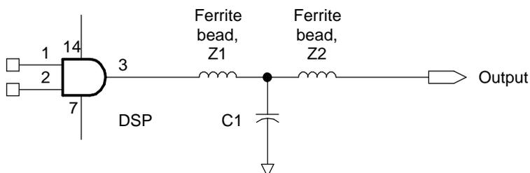
**Figure 4-16. Pi Filter Circuit for Power Supply Isolation**
