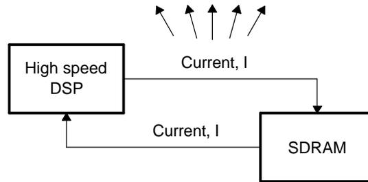
Differential mode radiation is directly related to the length of the signal trace, the driving current and the operating frequency. The electric field caused by differential mode radiation is
