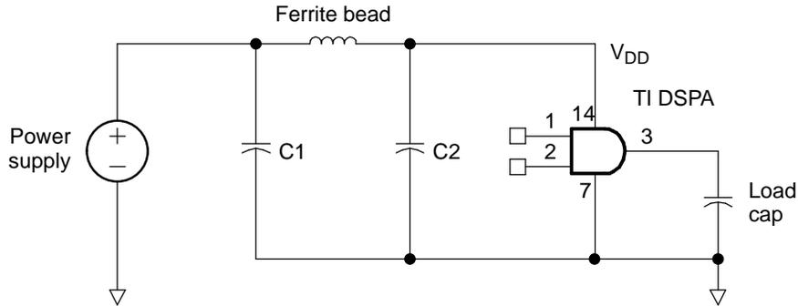
The filter bandwidth is calculated as follows:
