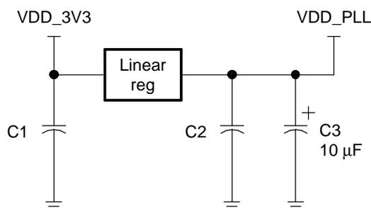
One method for low frequency filtering is shown in [Figure 6-10](#) where a resistor R replaces the ferrite bead and a bulk capacitor C3 (10uF to 33uF) is added to the circuit. Low frequency noise is attenuated by the resistor R and the bulk capacitor C3. The resistor needs to be selected such that the voltage drop across the resistor is negligible. The PLL supply voltage must be within the specified limits for worst case PLL current consumption.
