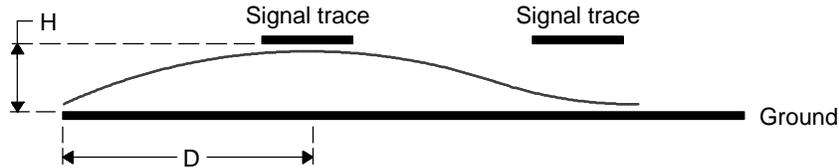
$$\text{Crosstalk} \approx \frac{K}{1 + \left(\frac{D}{H}\right)^2}, \text{ where } K \text{ is a constant less than } 1 \text{ and depends on the risetime and trace length}$$
