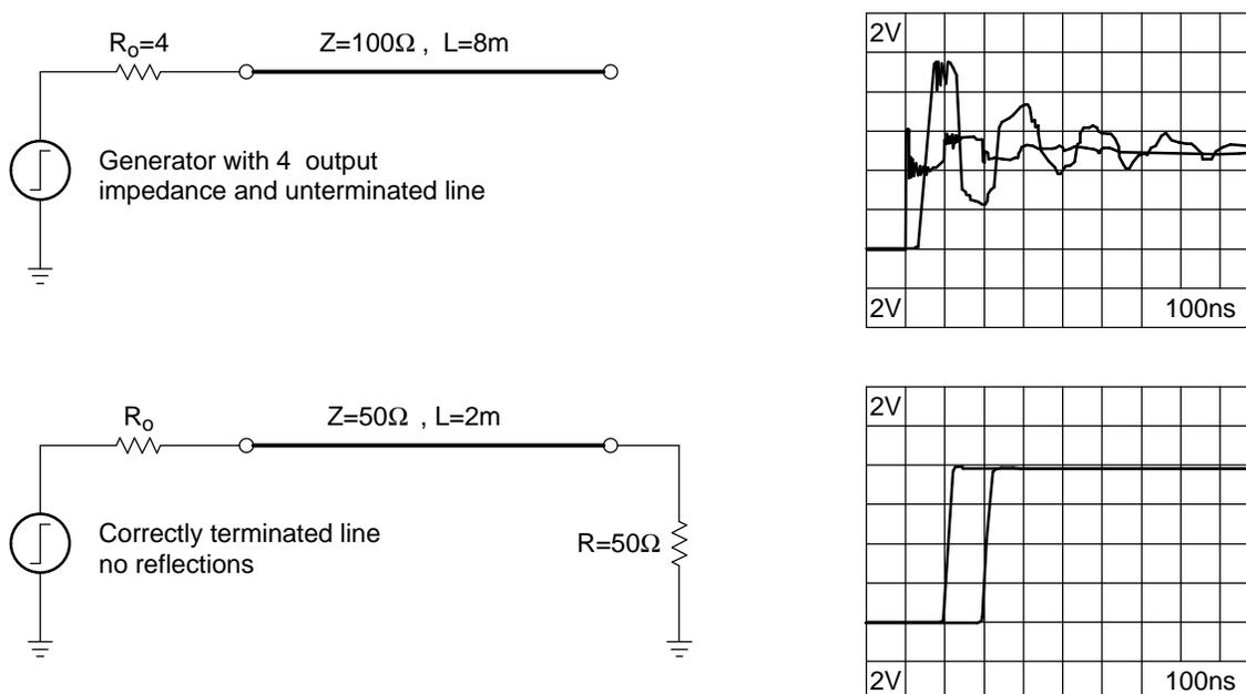
Figure 2-5. Parallel Termination Technique
