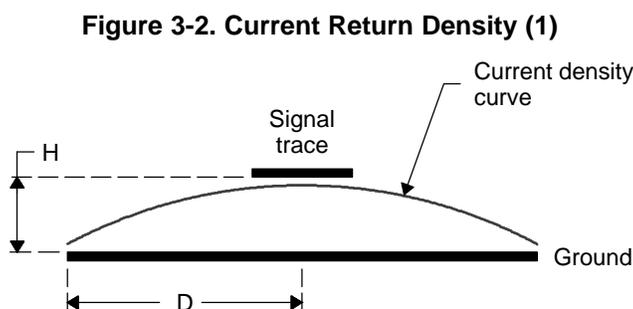
$$\text{Return current density} = I(D) = \frac{I_0}{\pi H} \frac{1}{1 + \left(\frac{D}{H}\right)^2}$$
