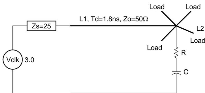
Figure 2-5 shows a parallel termination technique. This method can be used in the application where one output drives multiple loads as long as the traces to the loads called L2 are a lot shorter than the main trace L1.
