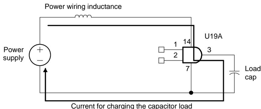
In Figure 4-5, the DSP labeled U19A is driving a capacitive load and is switching at a fast rate. Now, let us assume that the regulator is placed 5 inches away from the DSP and is routed with a 5 mil trace to the DSP. During fast switching, the power supply trace becomes an open circuit because of the parasitic inductance associated with the trace. This generates a large voltage droop at the pin of the DSP which can be estimated as follows.
