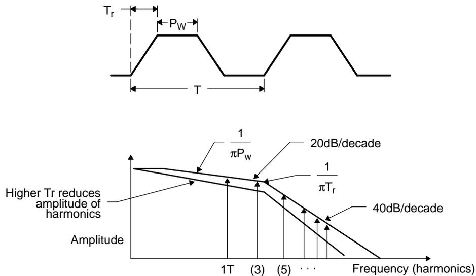
In [Figure 7-5](#), assuming a 50% duty cycle signal where only odd harmonics are present, the amplitudes of the harmonics decay slowly as frequency increases. The first pole frequency is at
