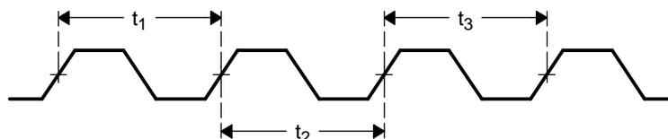
In [Figure 6-4](#), the cycle-to-cycle is measured by subtracting  $t_2$  from  $t_1$ ,  $t_3$  from  $t_2$ , and so on.
