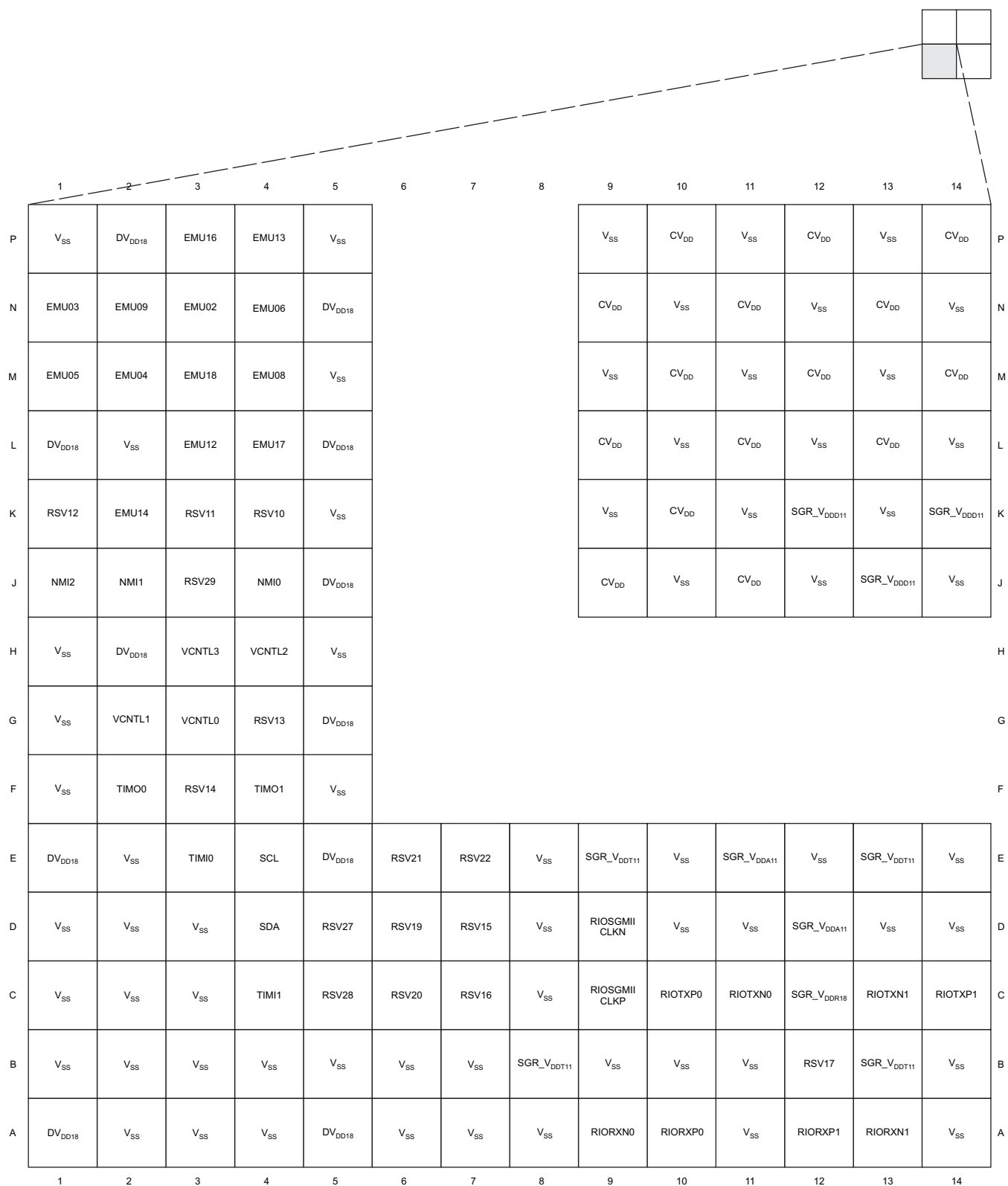
Figure 2-5. C6474 Pin Map (Bottom View) [Quadrant D]
