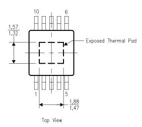
NOTE: All linear dimensions are in millimeters
