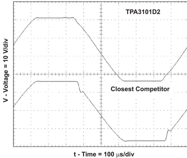
Figure 31. 1-kHz Sine Output at 10% THD+N
