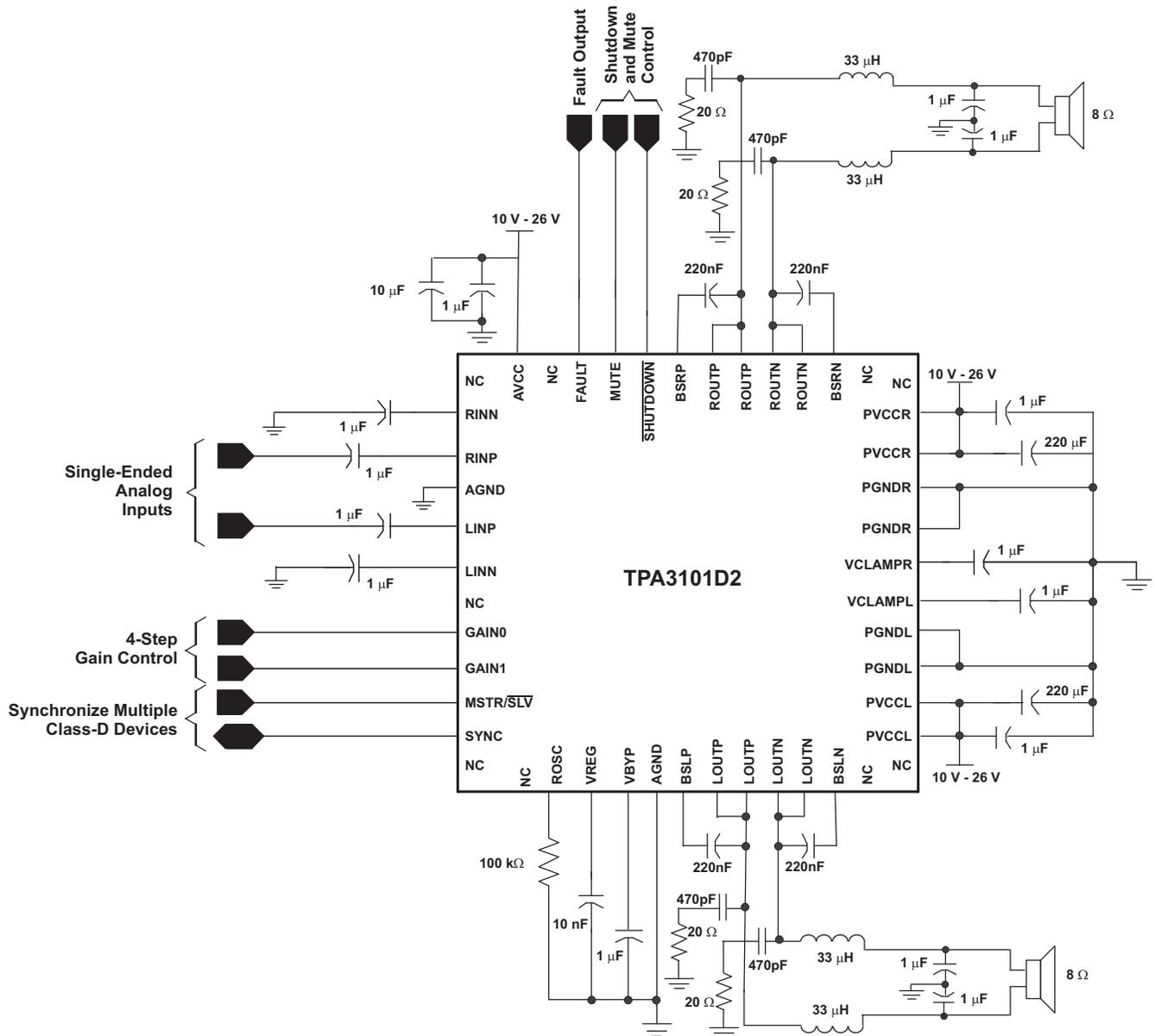
Figure 22. Stereo Class-D With Single-Ended Inputs (QFN)
