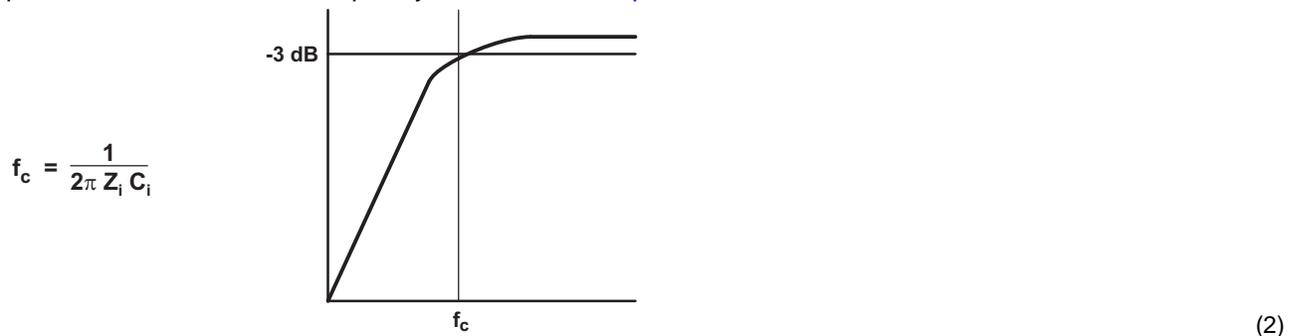
The value of  $C_i$  is important, as it directly affects the bass (low-frequency) performance of the circuit. Consider the example where  $Z_i$  is 20 k $\Omega$  and the specification calls for a flat bass response down to 20 Hz. Equation 2 is reconfigured as Equation 3.
