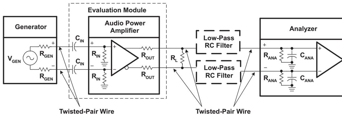
**Figure 36. Differential Input, BTL Output Measurement Circuit**
