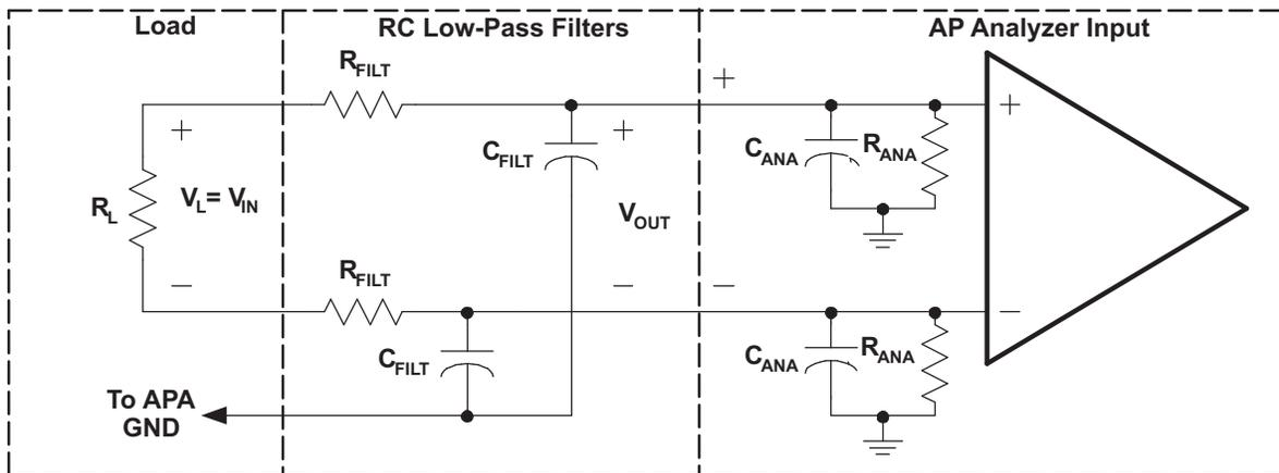
Figure 37. Measurement Low-Pass Filter Derivation Circuit-Class-D APAs
