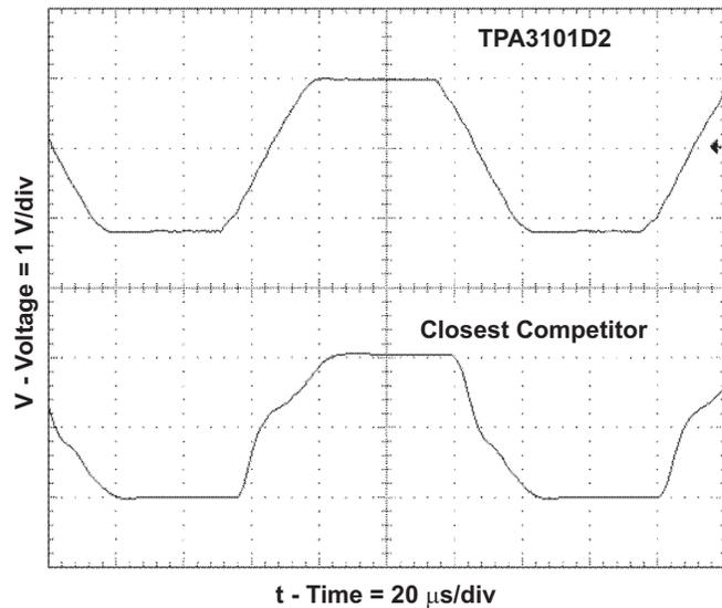
Figure 32. 8-kHz Sine Output at 10% THD+N
