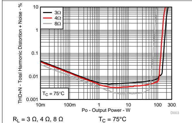
Figure 3. Total Harmonic Distortion + Noise vs Output Power
