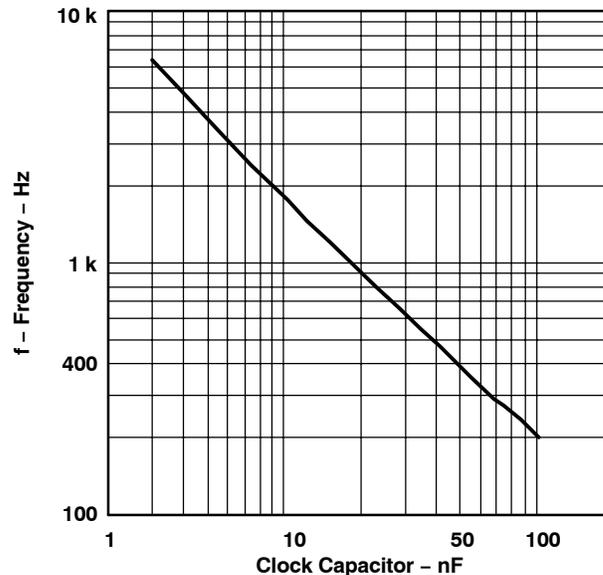
Figure 15. Clock Frequency vs Capacitance on Clock Pin
