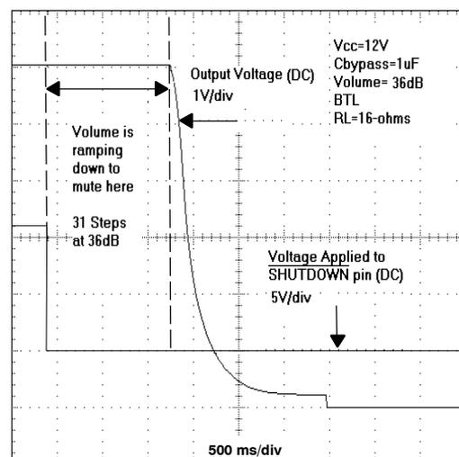
**Figure 18. Shutdown Curve When the Volume = 36 dB**
