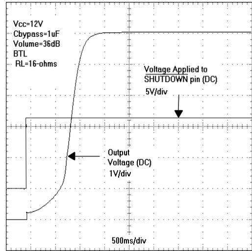
**Figure 20. Start-Up Curve When the Volume = 36 dB**
