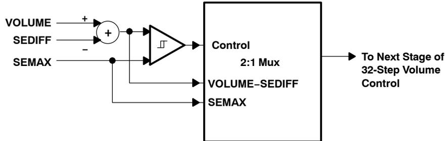
Figure 1. Block Diagram of the SE Volume Control
