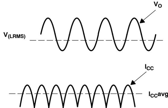
**Figure 27. Voltage and Current Waveforms for BTL Amplifiers**
