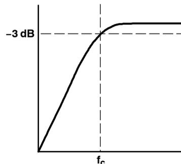
Large values of  $C_C$  are required to pass low frequencies to the load. Consider an example where  $C_C$  is 220  $\mu\text{F}$ , and the load varies from 16  $\Omega$ , 32  $\Omega$ , 10 k $\Omega$ , and 47 k $\Omega$ . Table 3 summarizes the frequency response characteristics of each of the preceding configurations.
