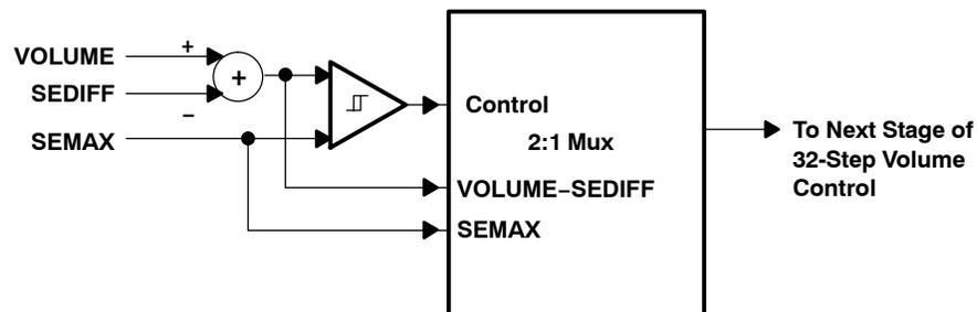
Figure 14. Block Diagram of the SE Volume Control
