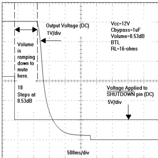
**Figure 17. Shutdown Curve When the Volume = 0.53 dB**
