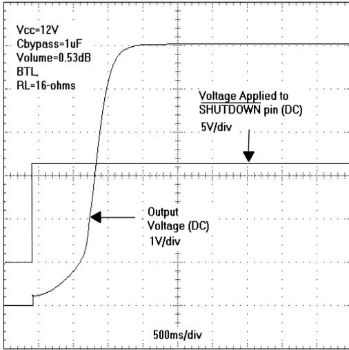
**Figure 19. Start-Up Curve When the Volume = 0.53 dB**
