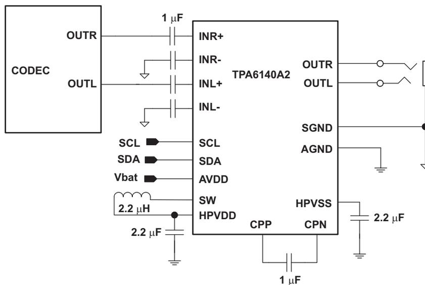
Figure 28. Typical Apps Configuration with Single-Ended Input Signals
