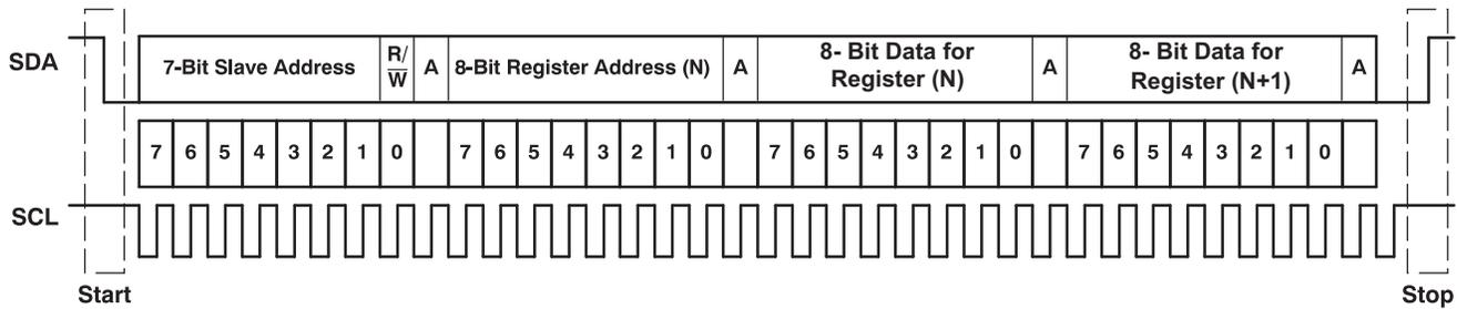
Figure 32. Typical I<sup>2</sup>C Sequence
