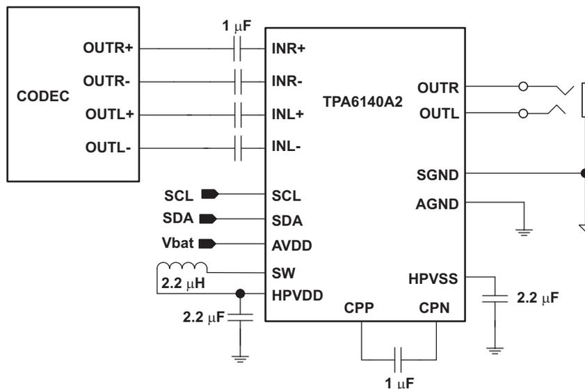
Figure 27. Typical Apps Configuration with Differential Input Signals
