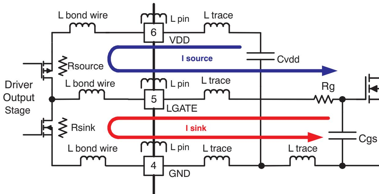
Figure 23. MOSFET Drive Paths and Main Circuit Parasitics
