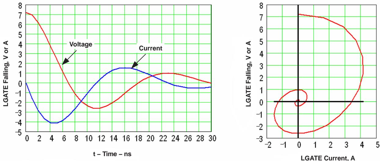
Figure 24. LGATE Turning Off Voltage and Sink Current vs Time (Related Switching Diagram (right))
