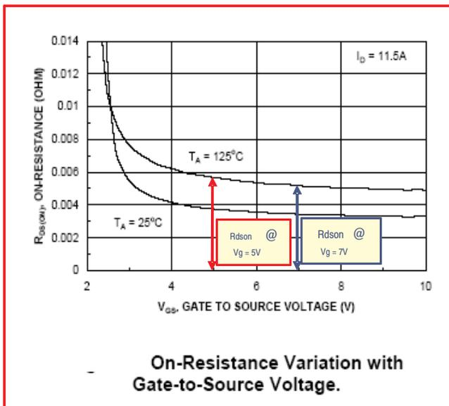
Figure 35.  $R_{DS(on)}$  of MOSFET as Function of  $V_{GS}$
