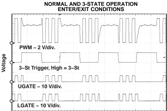
Figure 18. The 3-state upper threshold reverts to the 2-V level after the TPS28226 had been in 3-state for about 2.5  $\mu\text{s}$ .
