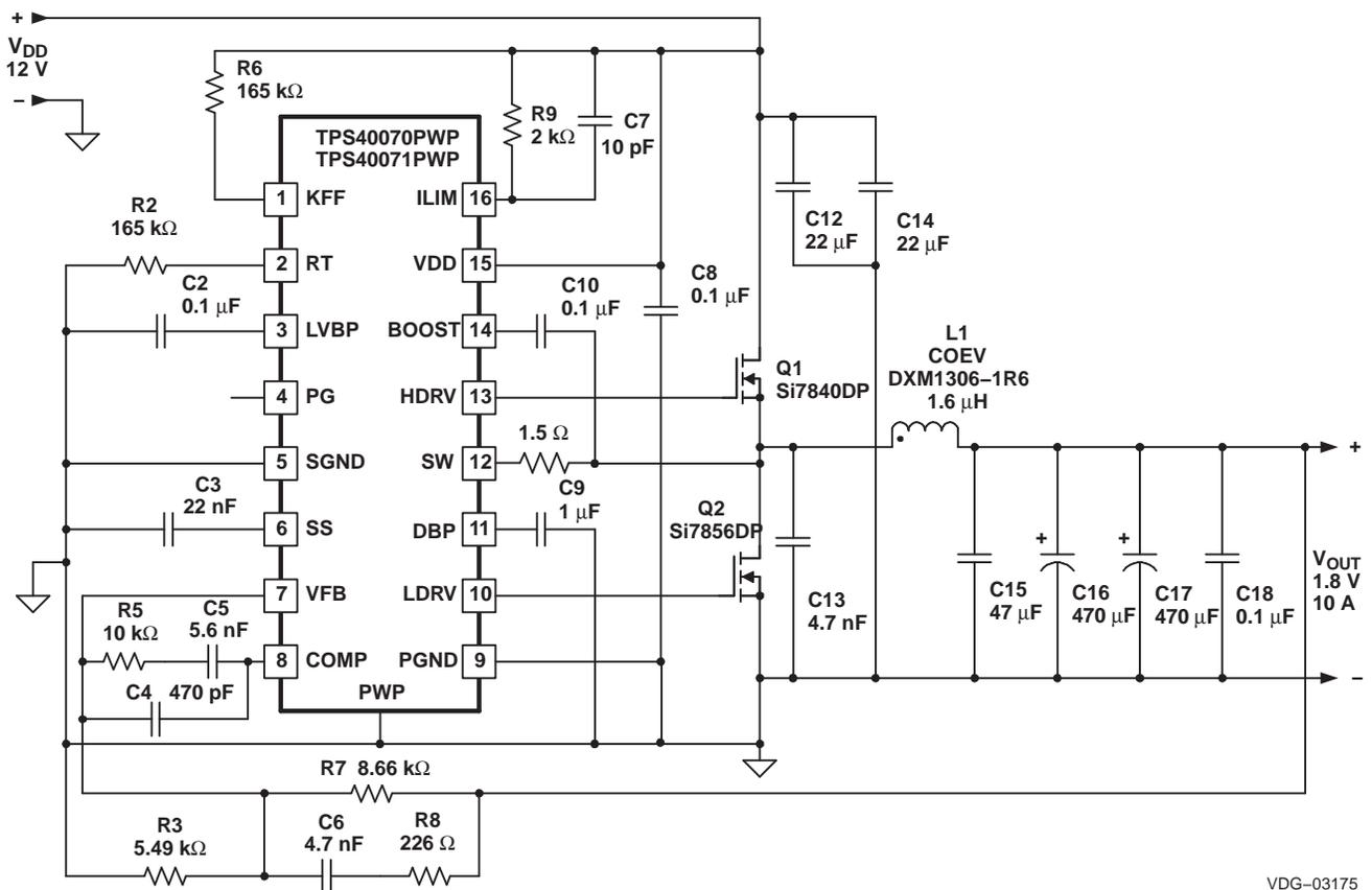
Figure 14. 300 kHz, 12 V to 1.8 V
