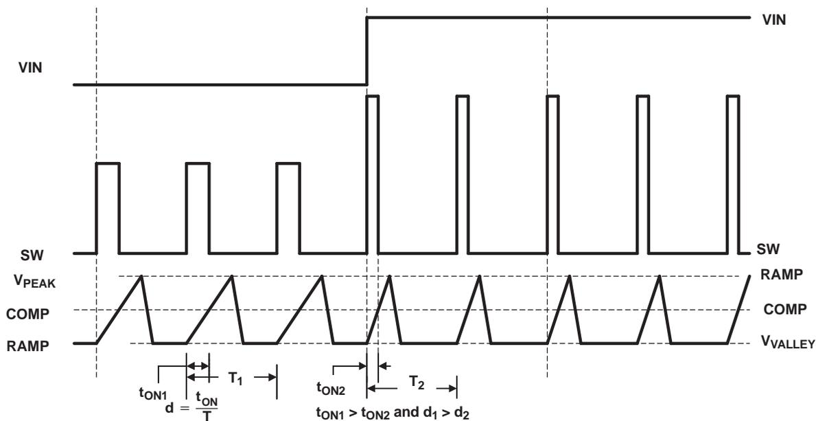
Figure 9. Voltage Feed-Forward and PWM Duty Cycle Waveforms
