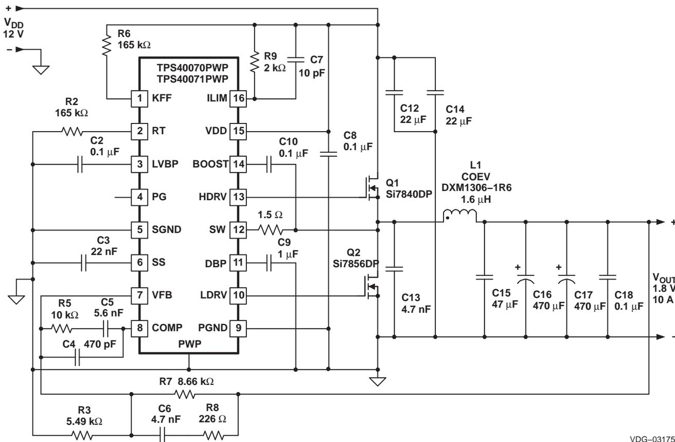
Figure 14. 300 kHz, 12 V to 1.8 V
