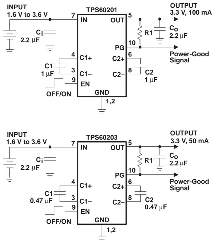
Figure 19. Typical Operating Circuit TPS60201 and TPS60203 With Power-Good Detector
