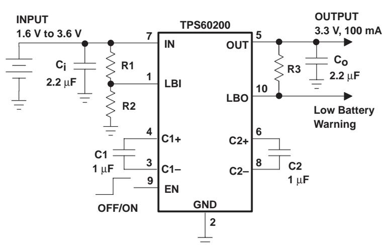
Figure 1. Typical Application Circuit With Low-Battery Warning
