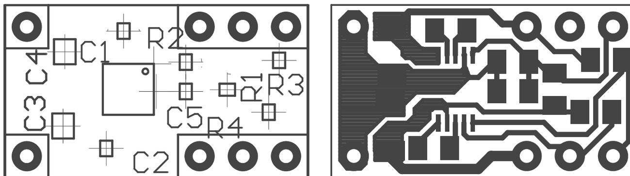
Figure 20. Recommended Component Placement and Board Layout
