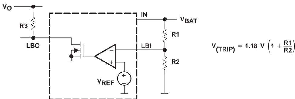
**Figure 2. Programming of the Low-Battery Comparator Trip Voltage**
