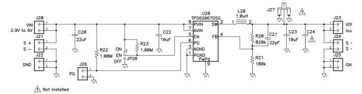
Figure 2. TPS62067EVM Schematic
