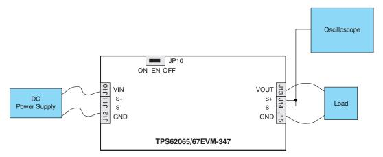
Figure 3. Hardware Board Connection
