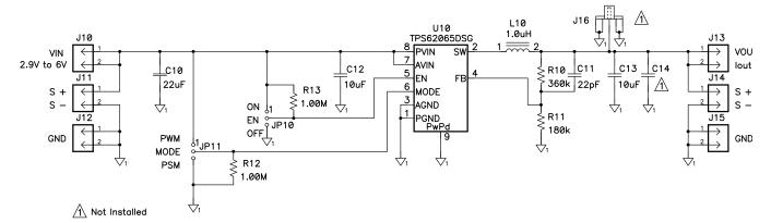
Figure 1. TPS62065EVM Schematic
