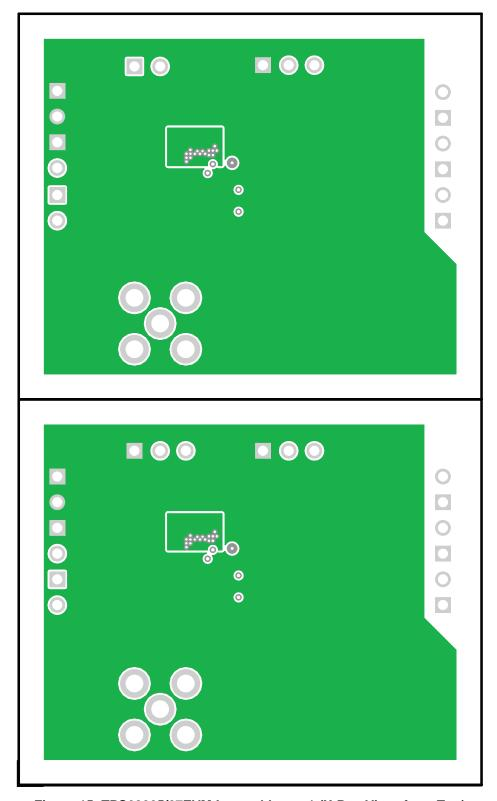
Figure 15. TPS62065/67EVM Internal Layer 1 (X-Ray View, from Top)
