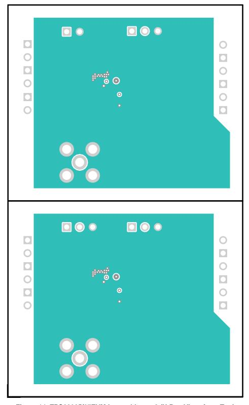
Figure 14. TPS62065/67EVM Internal Layer 2 (X-Ray View, from Top)
