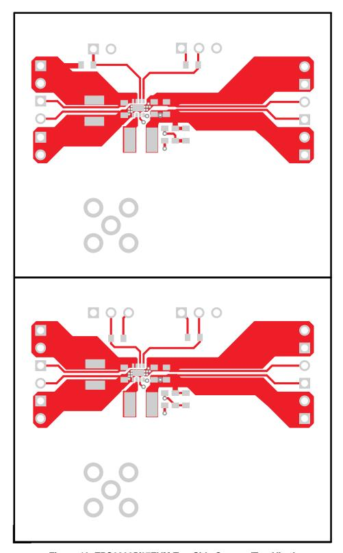
Figure 13. TPS62065/67EVM Top-Side Copper (Top View)
