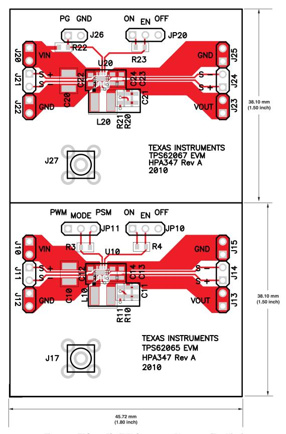
Figure 12. TPS62065/67EVM Component Placement (Top View)
