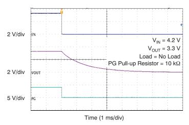
Conditions: VIN = 4.2 V,  $V_{OUT}$  = 3.3 V
