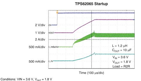
Figure 5. TPS62065 Startup into 2.2-Ω Load
