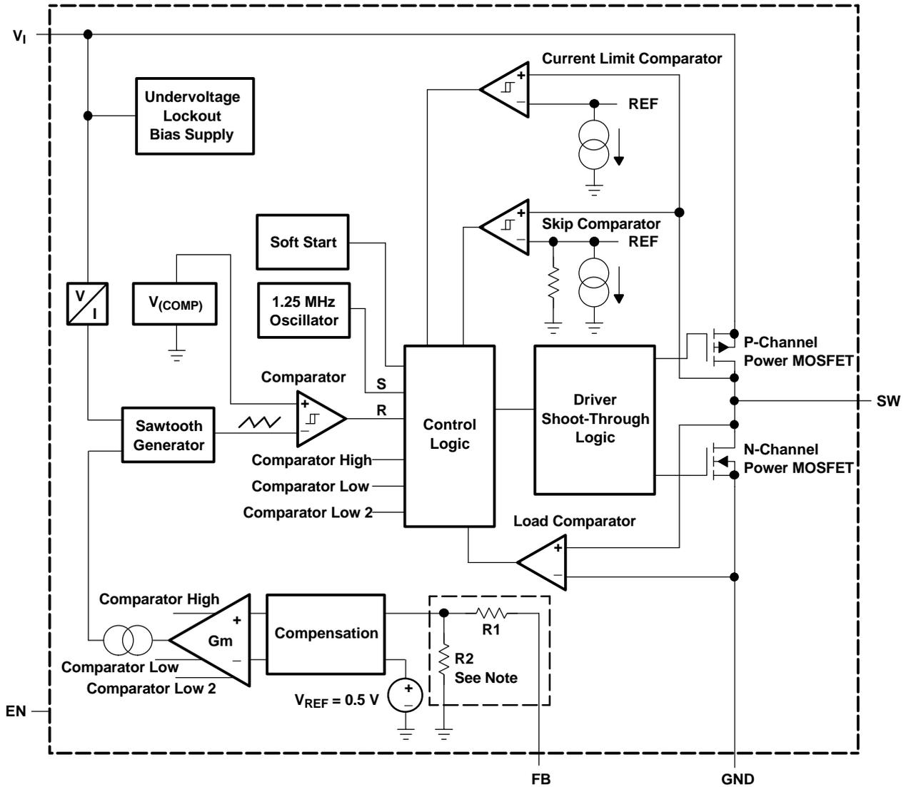
NOTE: For the adjustable version (TPS62220) the internal feedback divider is disabled, and the FB pin is directly connected to the internal GM amplifier
