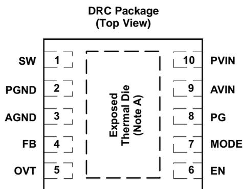
A. The exposed Thermal Die is connected to AGND.
