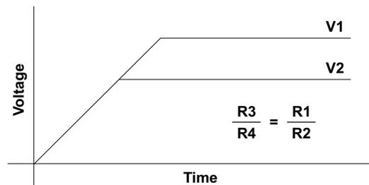
Figure 20. Simultaneous Tracking of V2 and V1
