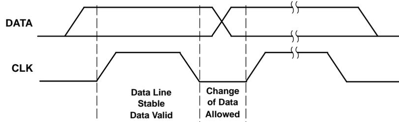
Figure 37. Bit Transfer on the Serial Interface
