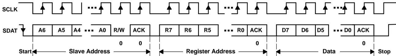
Figure 39. Serial Interface WRITE to TPS65012 Device
