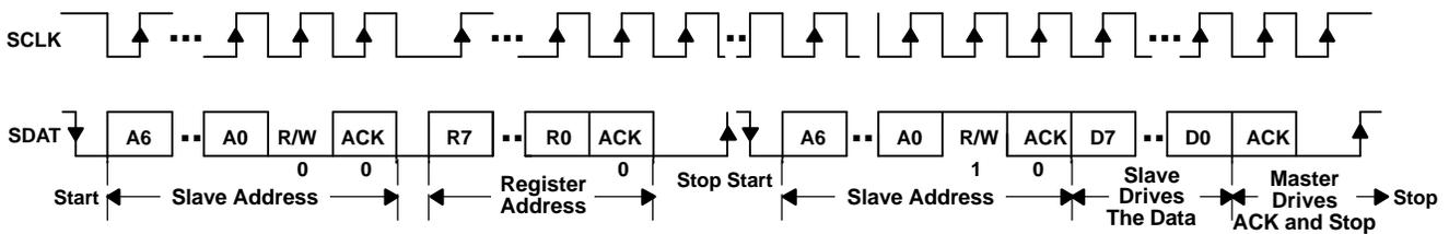
Figure 41. Serial Interface READ From TPS65012: Protocol B
