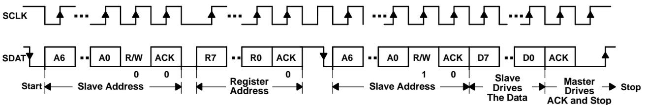
Figure 40. Serial Interface READ From TPS65012: Protocol A
