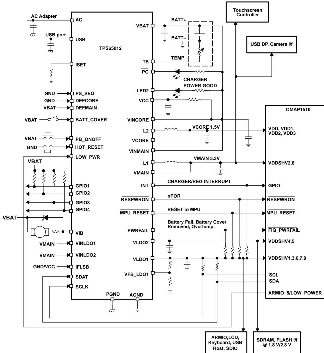
**Figure 44. Typical Application Circuit in Low Power Mode**
