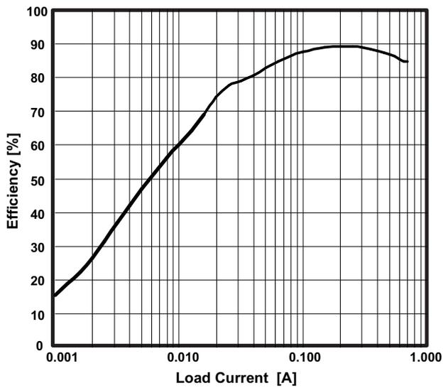
Figure 1. BOOST CONVERTER EFFICIENCY vs OUTPUT CURRENT
