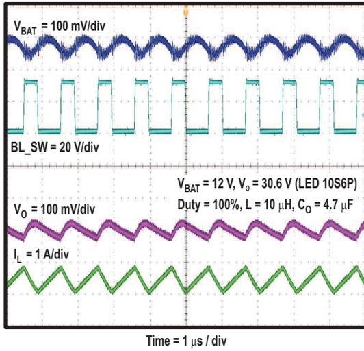
Figure 21. LED DRIVER SWITCHING WAVEFORM
