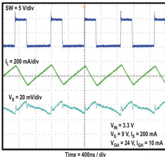
Figure 3. BOOST CONVERTER CONTINUOUS CONDUCTION MODE
