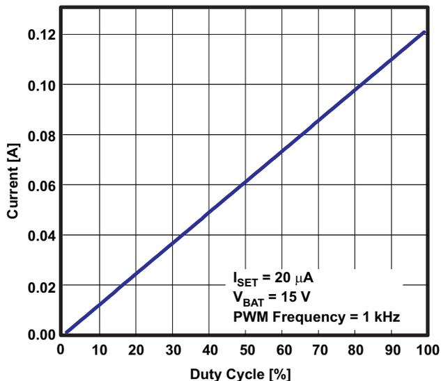
Figure 19. LED DRIVER PWM DIMMING LINEARITY 100Hz
