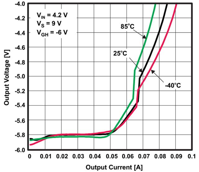
Figure 10. NEGATIVE CHARGE PUMP VOLTAGE vs LOAD CURRENT
