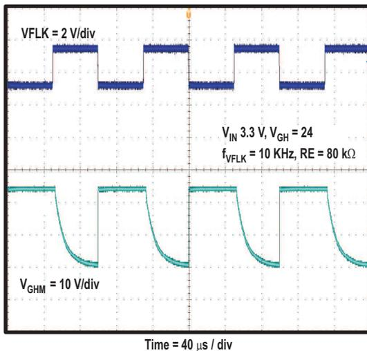
Figure 15. GATE VOLTAGE SHAPING
