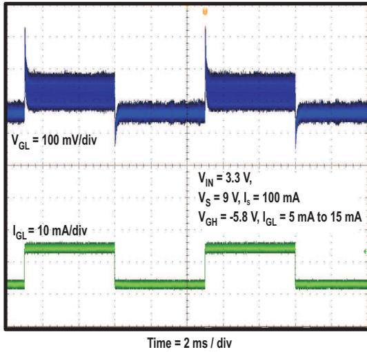
Figure 9. NEGATIVE CHARGE PUMP LOAD TRANSIENT RESPONSE
