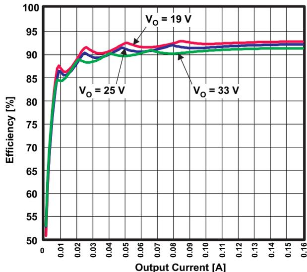
Figure 17. LED DRIVER EFFICIENCY vs OUTPUT CURRENT
