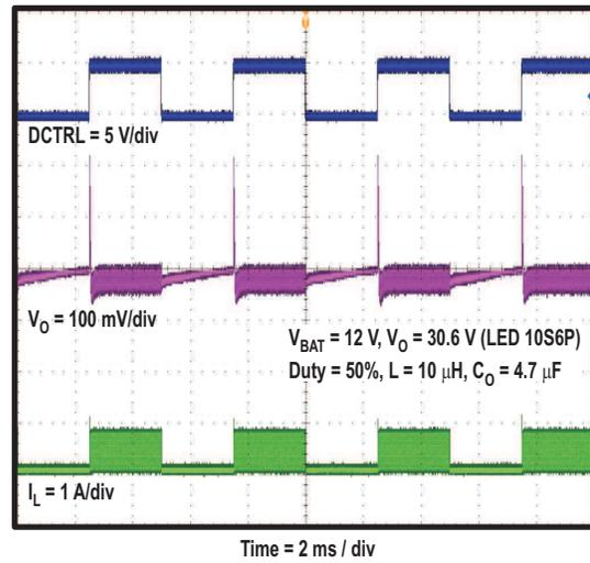
Figure 22. LED DRIVER OUTPUT RIPPLE AT PWM DIMMING
