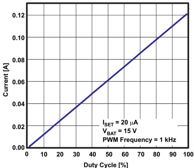
Figure 20. LED DRIVER PWM DIMMING LINEARITY 1kHz
