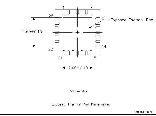
NOTE: All linear dimensions are in millimeters
