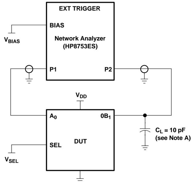
A.  $C_L$  includes probe and jig capacitance.
