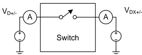
Figure 3. Off Leakage
