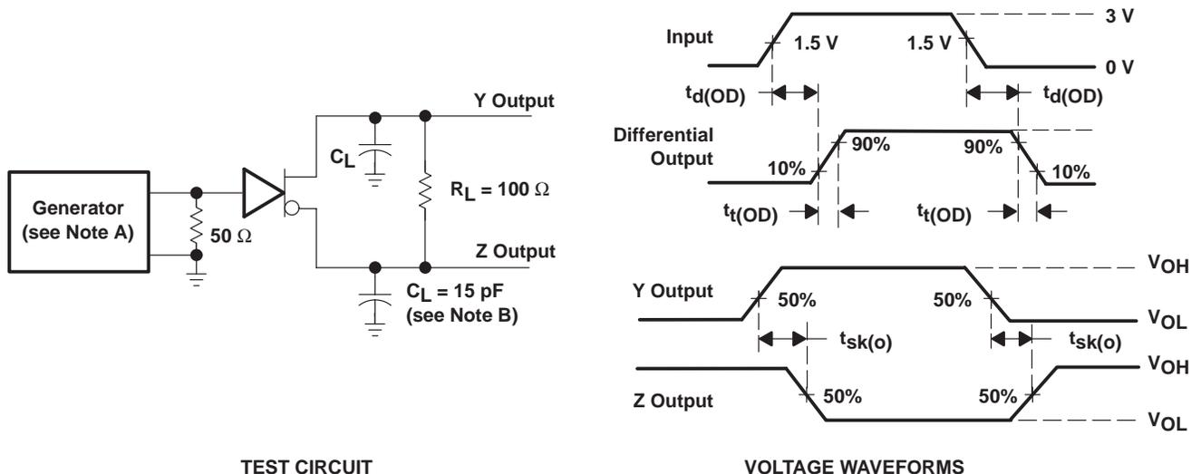
NOTES: A. The input pulse generator has the following characteristics:  $Z_O = 50 \Omega$ ,  $PRR \leq 500 \text{ kHz}$ ,  $t_W = 100 \text{ ns}$ ,  $t_r = \leq 5 \text{ ns}$ .
