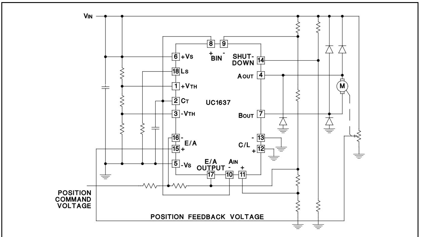
Figure 8. Single Supply Position Servo Motor Drive
