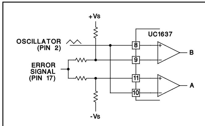
Figure 2. Comparator Biasing
