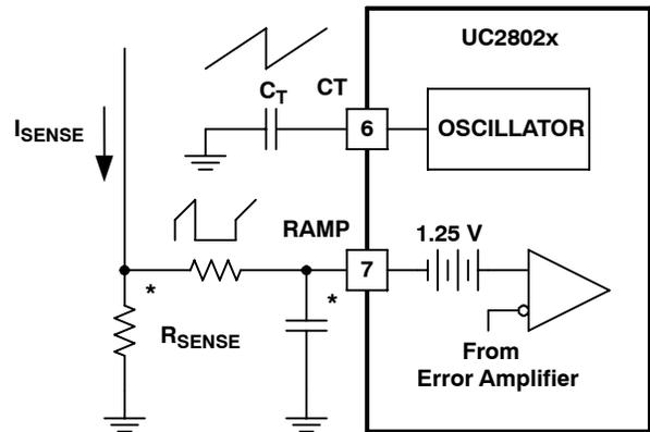
\* A small filter may be required to suppress switch noise.
