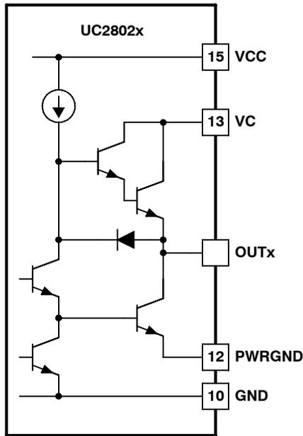
Figure 16. Simplified Schematic
