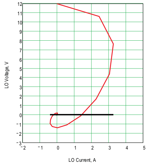
Figure 25. Turn-Off Voltage and Current Switching Diagram
