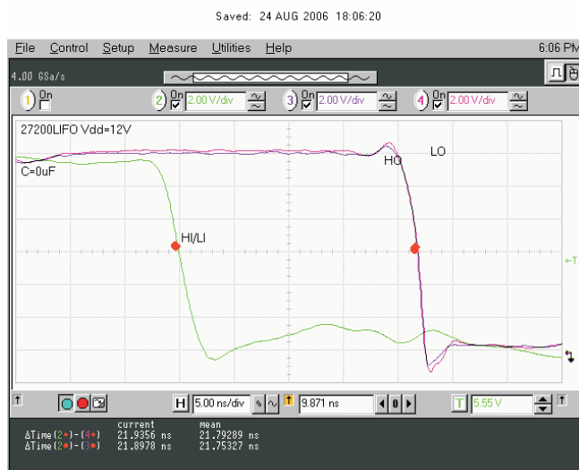
Figure 32. V_{LO} and V_{HO} Falling Edge Delay Matching
