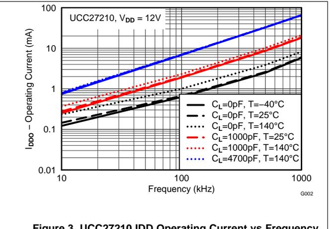
Figure 3. UCC27210 IDD Operating Current vs Frequency
