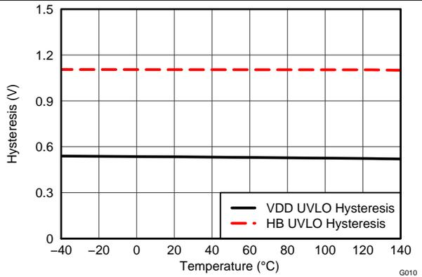
Figure 11. Undervoltage Lockout Threshold Hysteresis vs Temperature
