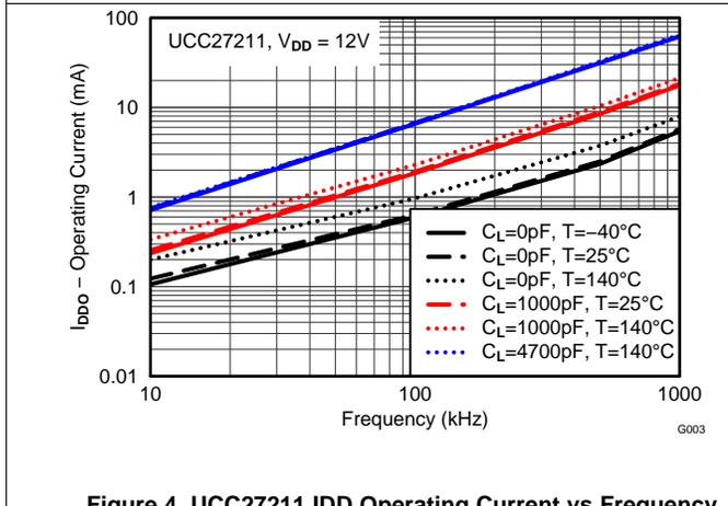
Figure 4. UCC27211 IDD Operating Current vs Frequency
