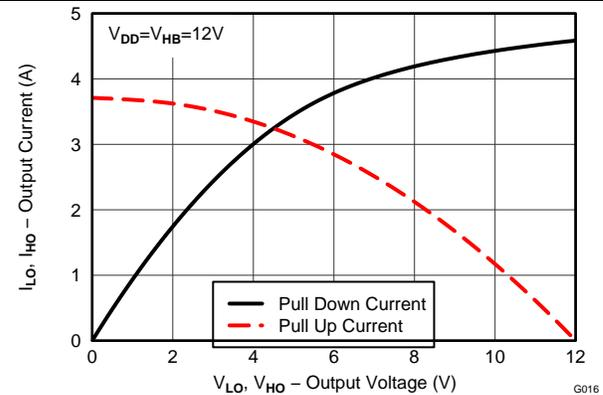
Figure 17. Output Current vs Output Voltage
