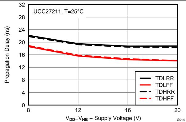
Figure 15. UCC27211 Propagation Delays vs Supply Voltage
