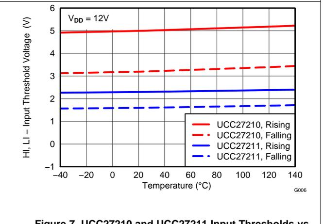
Figure 7. UCC27210 and UCC27211 Input Thresholds vs Temperature
