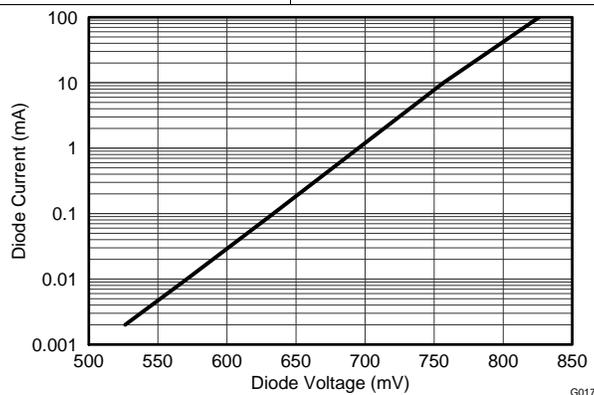
Figure 18. Diode Current vs Diode Voltage
