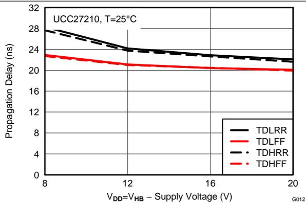
Figure 14. UCC27210 Propagation Delays vs Supply Voltage
