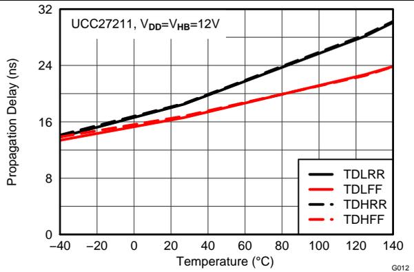
Figure 13. UCC27211 Propagation Delays vs Temperature
