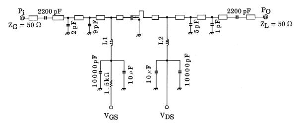
L1 :  $\phi 0.6 \text{ mm}$ , 5.5 mmID, 4T L2 :  $\phi 0.6 \text{ mm}$ , 5.5 mmID, 8T
