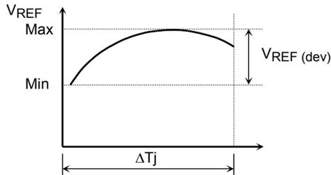
$$|\alpha V_{REF}| = \frac{\left( \frac{V_{REF (dev)} \times 10^6}{V_{REF @ 25^\circ C}} \right)}{\Delta T_j} \text{ (ppm/}^\circ\text{C)}$$
