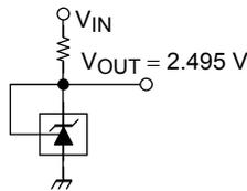
**(2) Shunt Regulator ( $V_{KA} > V_{REF}$ )**
