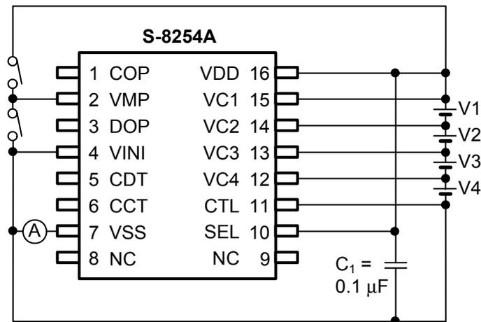
**Figure 4 Test Circuit 1**
