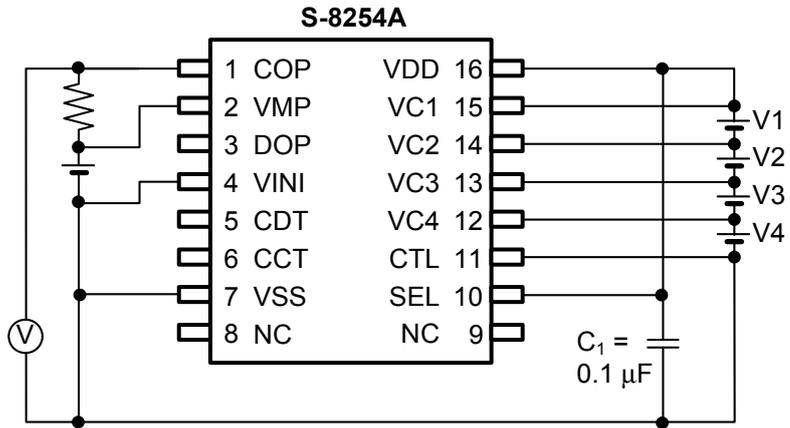
**Figure 7 Test Circuit 4**
