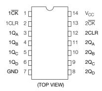
The TC74AC393 is an advanced high speed CMOS DUAL BINARY COUNTER fabricated with silicon gate and double-layer metal wiring C<sup>2</sup>MOS technology.
