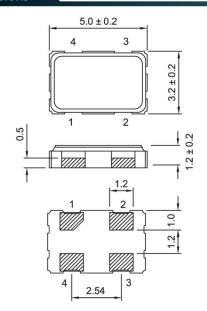
PAD FUNCTION: 1:ENABLE CONTROL 2:GND 3:OUT 4:VDD
