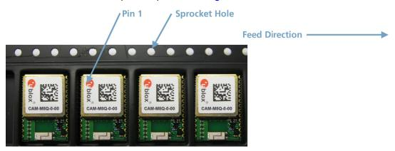
Figure 5: Tape and module orientation
