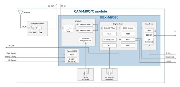
Figure 1: CAM-M8Q/C block diagram
