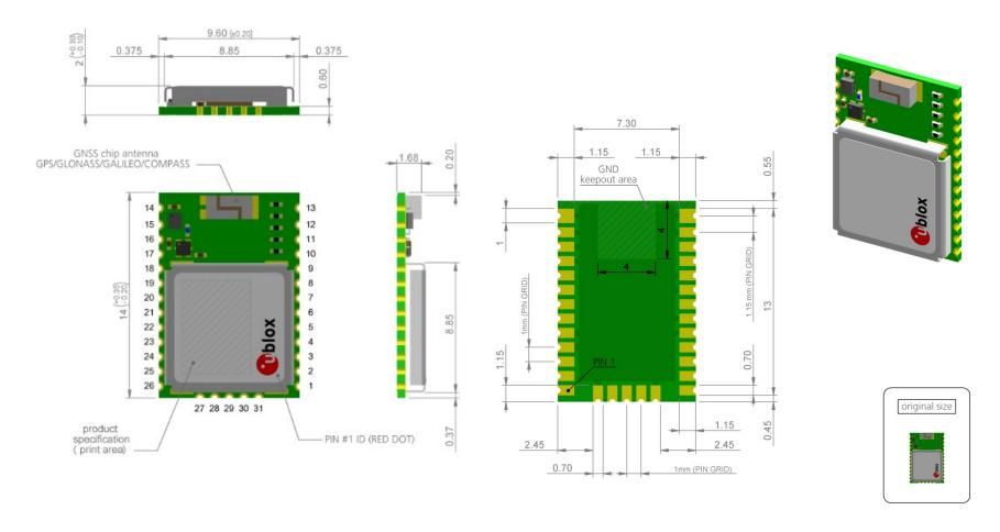
Figure 4: Dimensions (units: mm)
