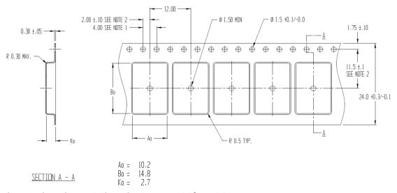
Figure 6: Dimensions and orientation for CAM-M8Q/C modules on tape
