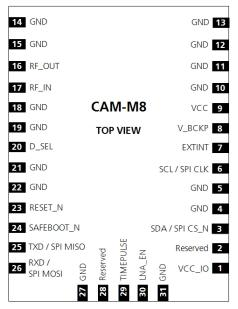
Figure 3: Pin assignment of CAM-M8Q/C
