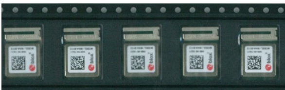
Figure 11: Orientation of NINA-W102/NINA-W106 module on tape
