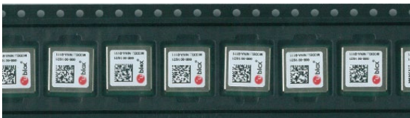
Figure 10: Orientation of NINA-W101 module on tape
