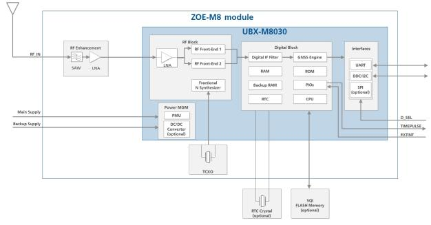
Figure 1: ZOE-M8 block diagram
