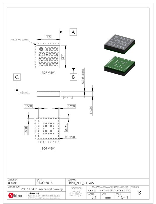
Figure 5: Mechanical drawing for ZOE-M8 (S-LGA), bottom view
