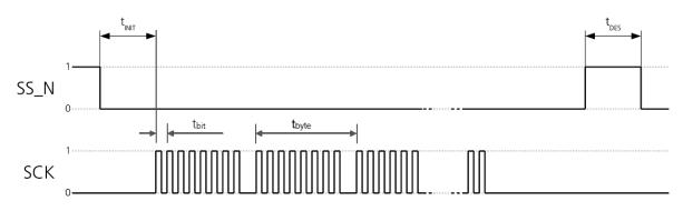
Figure 4: SPI timing diagram
