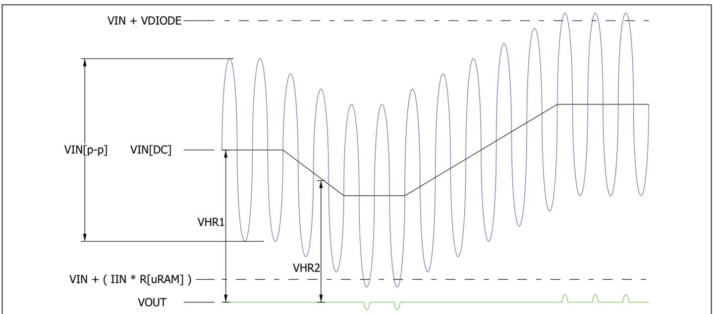
Figure 3 — Active Attenuation and the Effects of Headroom
