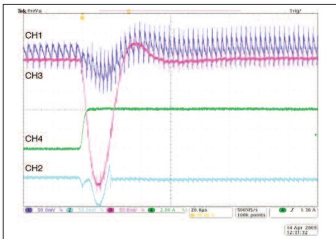
Figure 6 — Normal transient load response
