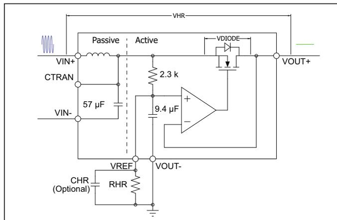
Figure 1 — Simplified MicroRAM Block Diagram
