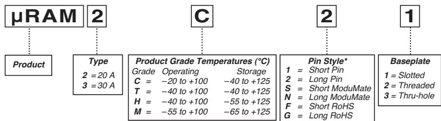
\*Pin styles S & N are compatible with the ModuMate interconnect system for socketing and surface mounting.
