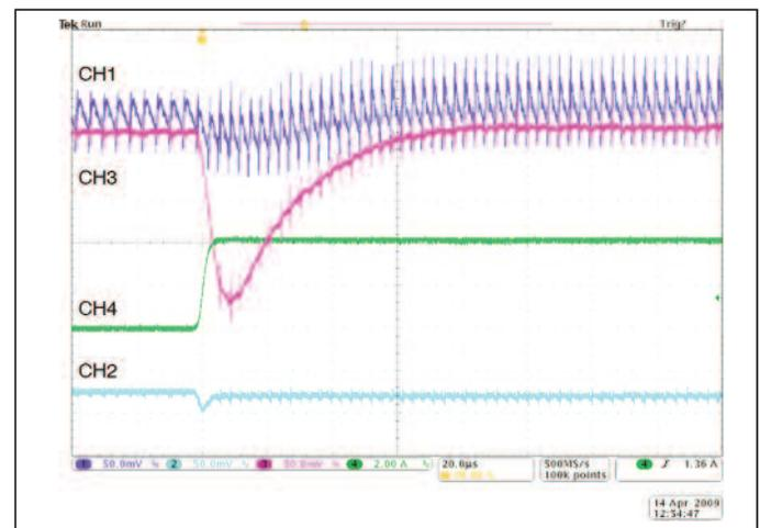
Figure 7 — Transient response with added CTRAN capacitor
