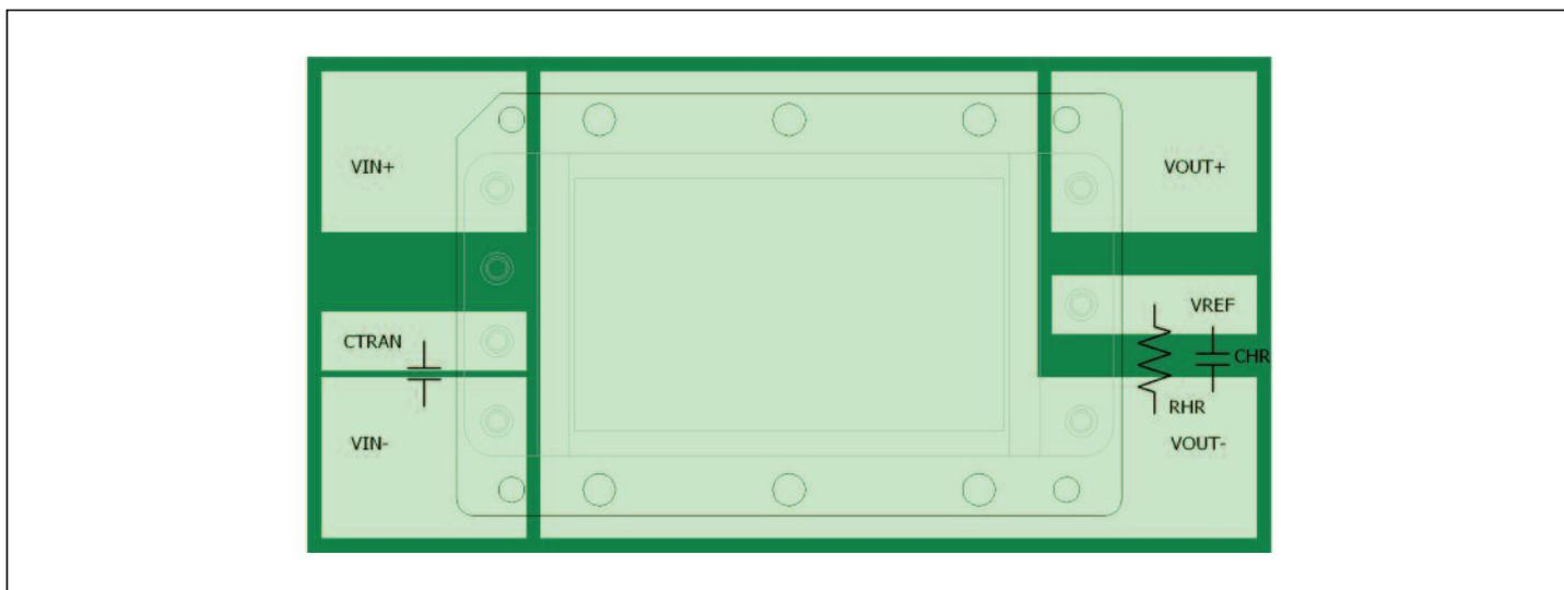
Figure 18 — Recommended copper patterns, top view.
