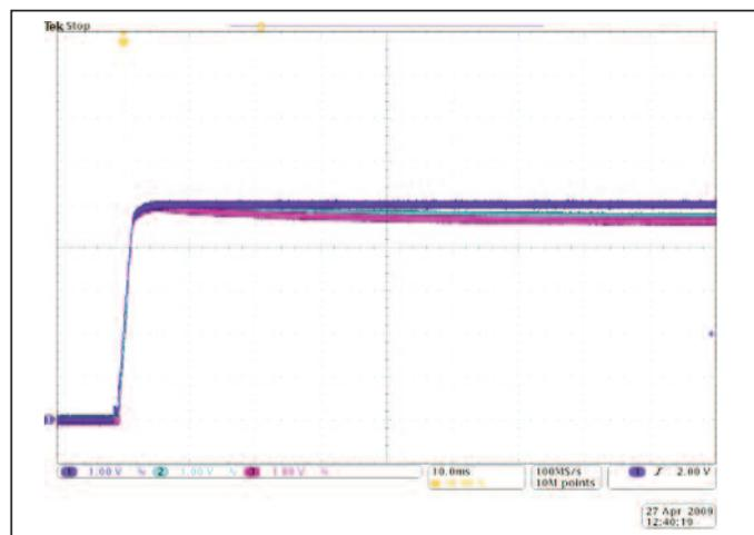
Figure 13 — Startup waveforms with the optional startup circuitry.
