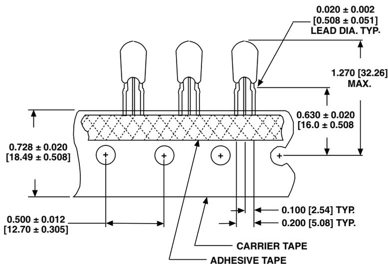
**Tape and Reel Specifications:** Type 299D radial-leaded tantalum capacitors are available taped and reeled per EIA-468.
