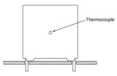
The temperature is measured in unloaded (T<sub>amb</sub>) and maximum loaded condition (T<sub>C</sub>).
