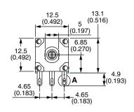
Single module, single shaft, vertical mounting, PC pins with support plate, metric bushing and shaft
