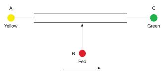
Direction of wiper displacement with shaft extended
