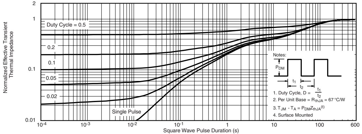
Normalized Thermal Transient Impedance, Junction-to-Ambient
