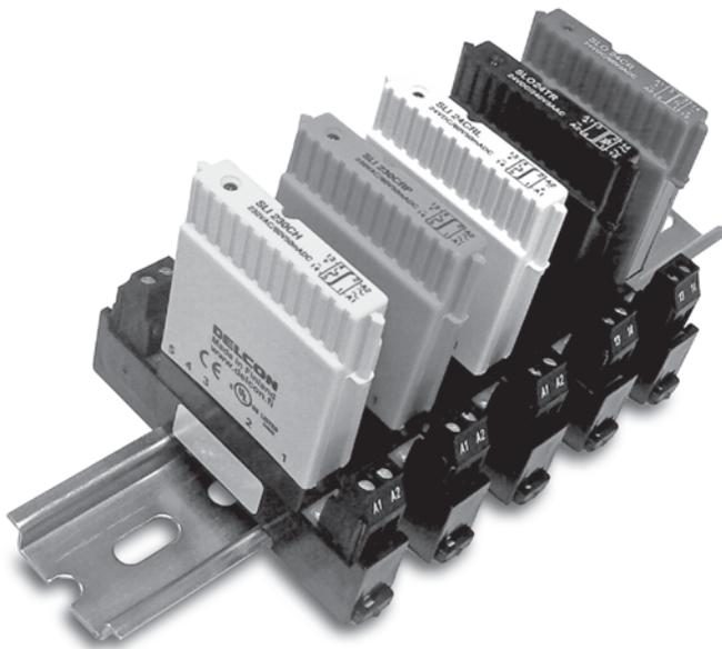
Pulse transformer technology for isolating I/O signals offers significant advantages over optical isolation and electromechanical relays. Most notably, pulse transformer I/O modules provide higher transient immunity and high input-to-output isolation.
