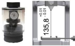
Verify that the press and the mini applicator's axis are perfectly in line.
