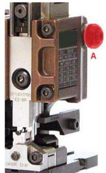
Manually cycle the press by means of a spanner until the terminal is positioned on the anvil. Loosen the nut A and turn the screw clockwise or counter-clockwise to determine the correct position. Then tighten the nut again and make a complete cycle of the press. If the result is not satisfying enough, repeat the operation.
