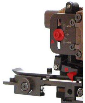
For adapting the pawl B to the pitch of the terminals, in order to have a new terminal correctly placed on the anvil for each cycle of the press: loosen the nut A and move the screw up for a greater pitch or down for a shorter one. Then tighten the nut again.
